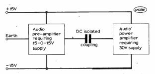
Fig. 6: Powering balanced and unbalanced equipment from a single supply.
