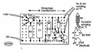
Fig. 2. The circuit can be constructed on veroboard as shown above. The board, transformer and neon lamp could be fitted into a suitable aluminium or plastic box.
