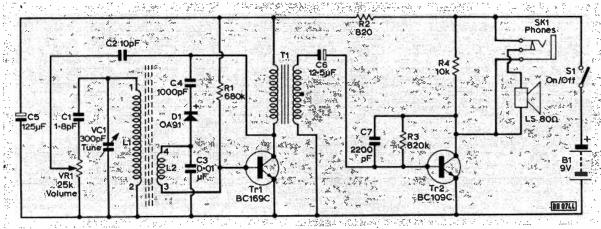
Fig. 1 : Circuit of the two transistor receiver.
