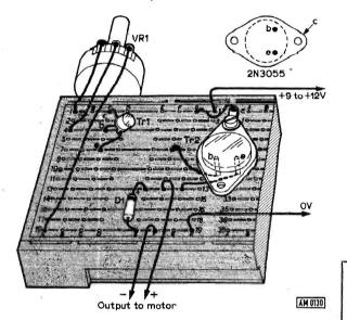
Fig. 39. Layout for Fig. 38. The short leads on Tr2 should be extended to connect to the T-Dec and the collector connection made via a solder tag bolted to Tr2.
