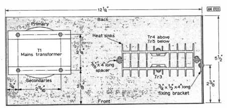
Fig. 9: Plan view showing mounting details of mains transformer and power transistor heatsinks.
