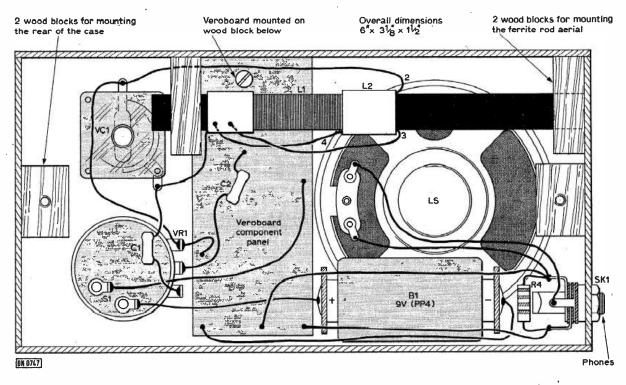
Fig. 4: General construction and layout details.
