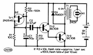
Fig. 1. Circuit of the neon flasher. R2, which, with C1, controls the flash rate could be made variable using a potentiometer. Additionally, C1 could have switched values.
