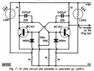
Interrupting the light to LDR2 restores the bistable so that Tr2 turns off. R8 may be altered to a lower value which will affect the sensitivity. It may be necessary to increase R6 and R7 to, say  $100k\Omega$  if low gain transistors are used.
