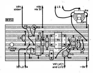
Fig. 3: Veroboard panel component layout.
