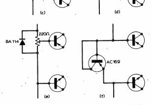
Fig. 1: (a) Basic complementary push-pull output stage, obtaining blas for the matched transistors from the voltage developed across diode. For germanium transistors, one silicon diode will develop the required p.d., but for silicon transistors, two silicon diodes in series will be necessary. Fig. 1 (b) to (f): Alternative methods of providing forward blas, showing typical values, exact values depending on transistors used and supply voltage.
