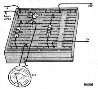
Fig. 35. Layout for Fig. 33. To carry out experiment in Fig. 34 change R2 to 10k $\Omega$  and insert R1.
