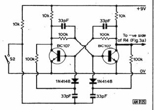
Fig. 6: Additional bistable switch circuit for long intervals, in place of \$4.
