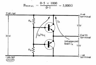
Fig. 4: Basic voltage divider using two emitter-followers.
