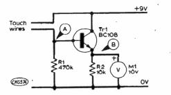
Fig. 34. The potential at A is set by the potential divide of R1 with skin resistance and this is reflected by the potential measured at B in the lower resistance emitter circuit.
