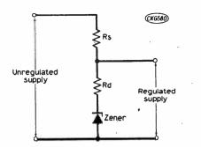
Fig. 3: Circuit of a perfect zener diode with a series resistance approximates the zener diode in practice.
