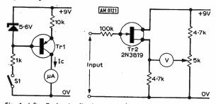
Fig. 1, left: Basic circuit of a constant-current generator. Fig. 2, right: Circuit of high impedance voltmeter.
