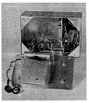
Capacitor C3 is held by a clip to the bottom of the box. A smaller' sized capacitor could be fitted inside the box.
