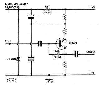
Fig. 5: AF pre-amplifier used in the GEC/Sobell range of portables forward biased by R82 directly from the collector, and applying both negative feedback and DC stabilisation.
