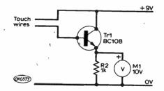
Fig. 33. The small current flowing through the fingers generates emitter current and this is shown as a potential difference across R2.
