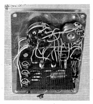
Photograph of prototype showing Veroboard bolted to front panel and interconnecting wiring.
