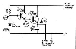
Fig. 40. A simple voltage dropper and regulator for running a cassette recorder from a car battery. Not short circuit protected.
