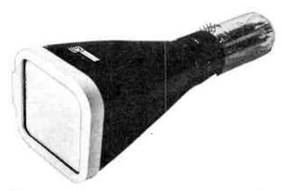
This E716A direct-view storage CRT is manufactured by the English Electric Valve Company has a viewing area of 10 × 10 cm. Because of its good deflection sensitivities it is particularly suitable for compact transistorised equipment. The normal storage time is from less than one second to several minutes but this can be extended to several days!
