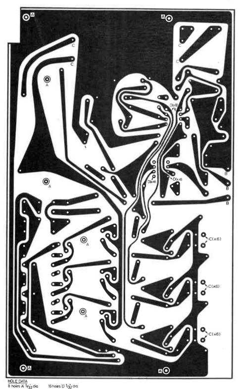
HOLE DATA 8 holes & 5/32 dia 3 holes B 1.8mm dia 22 holes C 1.3mm dia All other holes 1.0mm
