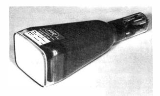
The Marconi-Osram Valve Company's 1400A single gun oscilloscope tube has a flat face with a display area of  $10 \times 8$  cm. The maximum final anode voltage is 4kV.
