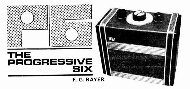
HIS portable receiver uses silicon n.p.n. epitaxial planar transistors in the first four stages, followed by a transformerless output stage employing germanium n.p.n. and p.n.p. complementary transistors. The circuit is relatively simple, while offering good sensitivity and adequate power output.
