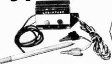
Have you ever built a project using digital IC's, only to find that it didn't work first time? The "Logiprobe" will enable you to see what is going on in TTL systems, giving a visual indication of the logic level at any point.
