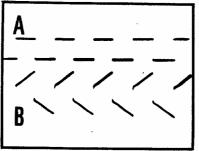
Fig. 25: Boosted I.f. response. A poorer amplifier may show some rounding of waveform B under similar conditions.
