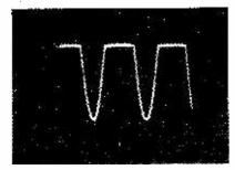
Fig. 4: Result of overloading the Y amplifier showing positive clipping.
