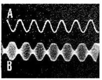
Fig. 19: 80 per cent modulation with some clipping.
