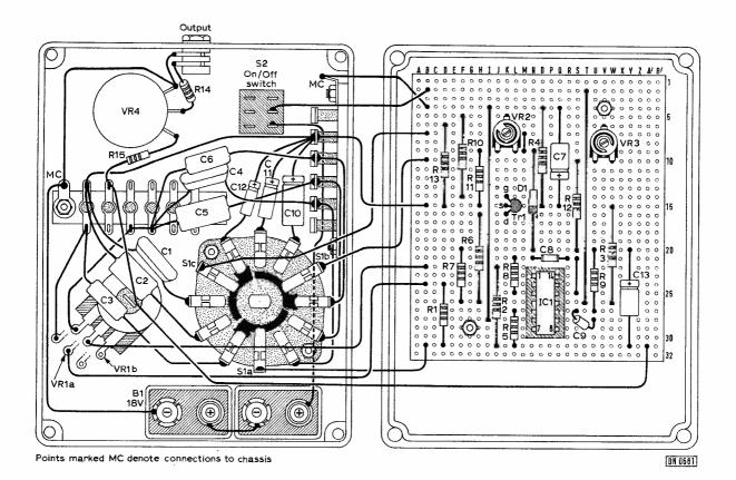
Fig. 3. The larger components are fitted in the die cast box, left, with the remaining components mounted on the lid, right.
