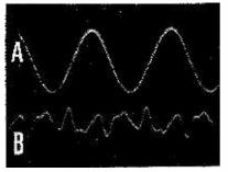
Fig. 33 : The distortion seen on the 50Hz mains.
