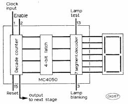
Block diagram of Motorola MC4050 i.c. which requires only the addition of a power supply and seven segment readout display for a complete decade counter.
