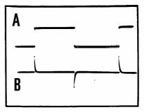
Fig. 8: Waveform A shows a square-wave while B shows the differentiated output.
