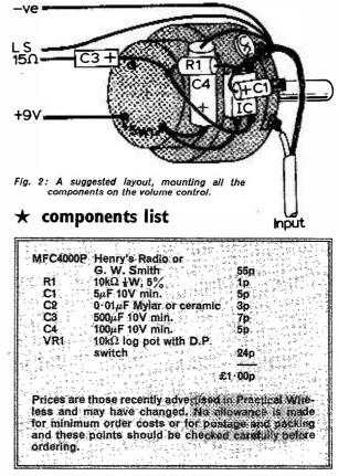
Quiescent current drain is only about 3.5mA, though this rises to 60mA or more on peaks and a substantial battery such as a PP9 is needed to drive the unit. The power supply described in the last *Take 20* can also be used.
