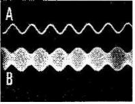
Fig. 18: A shows a sine-wave, B shows the same signal modulating an r.f. carrier to about 50 per cent.
