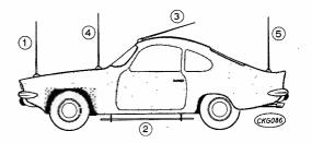
Fig. 1: The various possible positions for the car radio aerial.
