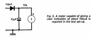
To do this, the test set-up of Fig. 5 is required to monitor the output of ICl. S1 is set to the middle range and VR1 to mid travel. With VR3 in its extreme anti-clockwise position, advance it slowly until the meter starts to indicate. Further advancement will give a rising meter reading which will start to level off as VR3 is rotated further; stop at this point.
