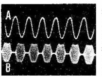
Fig. 20 : Greater than 100 per cent modulation resulting in top and bottom clipping.
