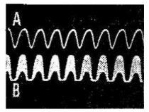
Fig. 22: A complex waveform due to stray coupling.
