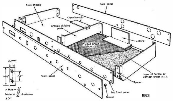
Fig. 46 : Exploded view of the metalwork. Note the addition of the three metal strip spacers introduced between the sub front panel and chassis. These have been introduced to facilitate easier mounting of the printed circuit board.
