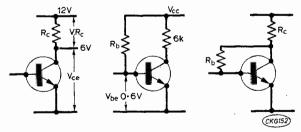
Fig. 47, left. Biasing, the first steps: determining collector voltage. Fig. 48, centre, the effect of the base bias resistor. Fig. 49, right, returning the "upper" end of R<sub>b</sub> to the collector considerably alters conditions.
