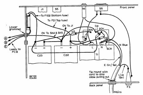
Fig. 45: Power supply wiring details and component positioning.
