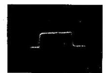
Fig. 3: Half a cycle of a 10kHz square-wave applied direct to a 'scope.
