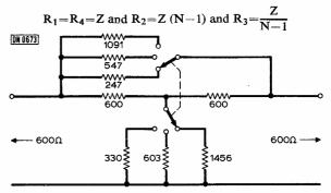
Fig. 5. Switched attenuator for 3, 6 or 9dB. A practical circuit would use preferred value resistors.
