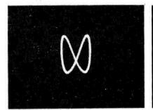
Fig. 13: A two-to-one Lissajous pattern.
