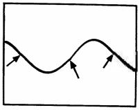
Fig. 29: Crossover distortion indicated by the arrows.
