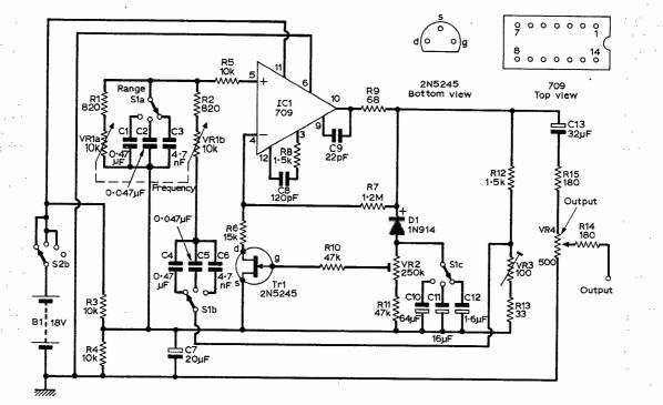
Fig. 1. Circuit of the simplified audio signal generator.
