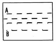
Fig. 23: A 1:1 square-wave as applied to an amplifier (A) and as seen at the output (B). The fastrisetime on the verticals means that this part of the waveform cannot be seen.
