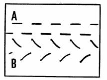
Fig. 24 : The applied signal (A), with the output (B), showing poor I.f. response.
