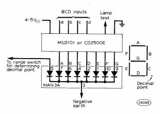
Decoder and driver functional diagram for operating the Monsanto MAN3A alpha-numeric display.
