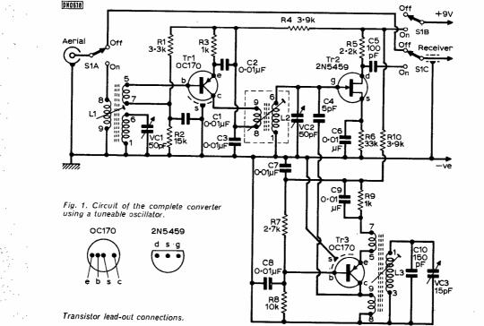
Fig. 2. Layout of the tuneable version of the converter. Tuning capacitor VC3 and associated components are not required in the crystal controlled version, shown in heading photograph.
