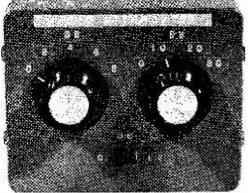
The die cast box carries all the components. The three switches provide any attenuation between 0 and 39dB.
