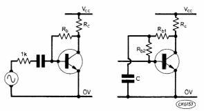
Fig. 50a, left, shows why the input resistance must be accounted for. Here the source is shown as a voltage generator with its resistance in series. Fig. 50b, right, shows how by "splitting" R<sub>b</sub> and decoupling the junction point, we can modify the feedback.
