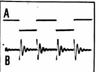
Fig. 28 : Severe ringing in an amplifier.
