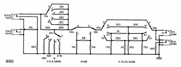
Fig. 6. Practical design for the attenuator illustrated, incorporating  $\pi$  and T pads.
