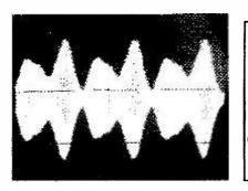
Fig. 36: Waveform from a rotating tremulant loudspeaker.
