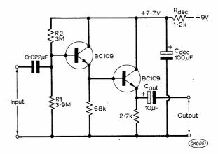
Fig. 45. Reproduction of Fig. 30, p.1008 of March PW, showing a Darlington pair, as previously described, with special attention in the text to the effect of the  $68k\Omega$  emitter resistor of the first transistor.
