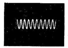
Fig. 1: A 1kHz sine wave illustrating good linearity.
