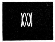
Fig. 15: A four-to-one frequency ratio.
