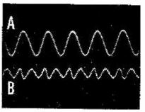
Fig. 32: Harmonic distortion. A shows the input while B shows the output with the fundamental signal removed.
