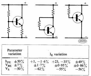
Fig. 51. Comparison of biasing arrangements, showing the effect of spreads of emitter current that can result from changes in hFE and VBE for alternative supply voltages. Nominal values of parameters are:  $V_S = 7V$ ,  $V_{BE} = 0.7V$ ,  $h_{FE} = 100$ ,  $I_E = 10A$  (approx.).
