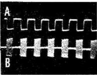
Fig. 21 : Gross over modulation resulting in squared pulses. Such a signal will produce severe harmonics.
