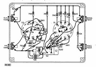
Fig. 7. Component layout. All resistors are  $\frac{1}{2}W$  5%, S1 is 2-pole 5-way, S2 is a 2-pole 2-way slide switch and S3 is 2-pole 4-way.
