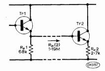
Fig. 46. Input resistances separately calculated for each section of a combined stage. This is not really a true picture, see text.
