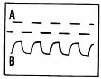
Fig. 26 : Poor h.f. response or full treble cut.
