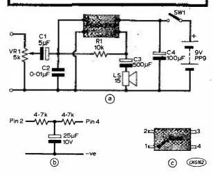
Fig. 1: (a) The complete circuit of the amplifier, (b) an alternative arrangement to replace R1 but see text, (c) the lead identification viewed from the top.
