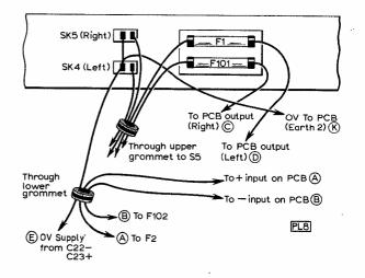
Fig. 44: Details of sockets SK4, SK5 and loudspeaker fuse mounting.
