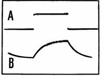
Fig. 35: The integration of a square-wave signal.
