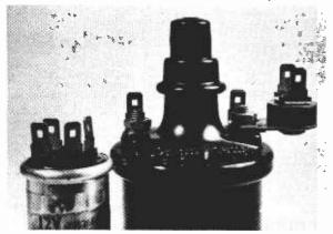
One version of "cold start" coil with button type carbon ballast resistor mounted on one terminal. Also shown is a typical relay which shorts out the ballast resistor on starting.
