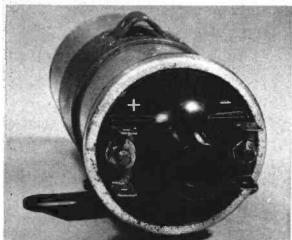
Standard ignition coil. Solder type tag connections should be replaced with push-on type connectors as shown, to facilitate reversion to normal Ignition system.
