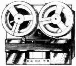
4-track record/playback head. Plus 4-track erase head. Positive pressure pad system. Takes any tape spool up to and including 7". The R.C. 74 is driven by a powerful 200/250V 50-cycle A.C. motor. A heavy, accurately balanced, flywheel brings wow and flutter levels down to approx. 0.3% total at  $3\frac{1}{4}$  and  $7\frac{1}{2}$  ips. Fast rewind in both directions.
