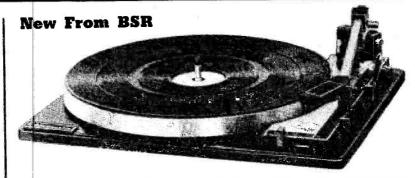
Leader of the three latest models from BSR is the BSR HT70 McDonald deck. It has all the features of the MP60 with three important developments: a heavier 514lb. deep rim turntable, a synchronous 4-pole dynamically balanced motor and a rotating record stub spindle to combat record drag.
