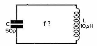
Fig. 1: A tuned circuit of which the resonant frequency is unknown.
