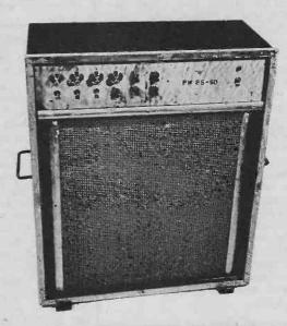
The completed Vibrasonic amplifier which utilises two 12in. speakers to handle the output of 50 watts (r.m.s.)
