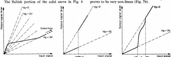
Fig. 6: The dashed lines on the graph show the audio stage gains at different f.e.t gate voltages for the circuit in Fig. 5.
