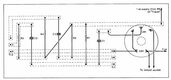
Fig. 2 : Full scale layout of the "generator" circuit board
