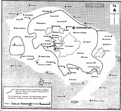
This v.h.f. service transmits on 95.6MHz, horizontal polarisation. Maximum e.r.p. is 5.5kW with a directional aerial.
