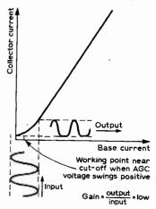
Fig. 2: Radio receiver a.g.c circuit and graphs showing effect of a.g.c on gain.
