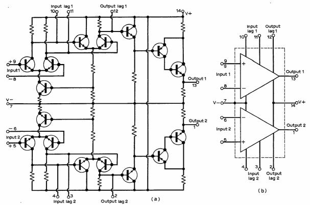
Left: Circuit of MC1303, stereo preamplifier unit. Right: Simplified diagram of the preamplifier.
