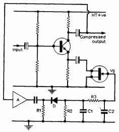
Fig. 5: The compressor circuit principle.
