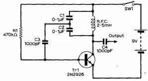
Fig. 1: The circuit diagram of the signal injector.
