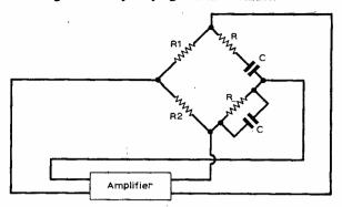
Fig. 5.5. Basic circuit of the Wien bridge oscillator
