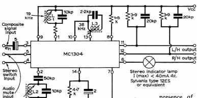
Left: The external circuitry required for full stereo decoder facilities using the MC1304. The righthand side of the indicator lamp goes to the 12V supply. Lefthand channel output is between pln 11 and earth and righthand channel output between pln 12 and earth. With a supply voltage of 12V the resistor at pin 8 should be changed to  $2.7 k\Omega$ .
