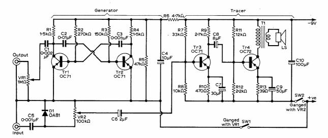
Fig. 1 : Circuit of the Genetracer. The "generator" and the "tracer" are built on separate circuit boards
