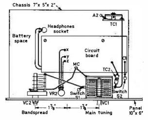
Fig. 4: Top view of chassis and circuit board.
