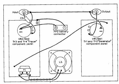
Fig. 4: Interconnection of the circuit boards after mounting in cabinet.
