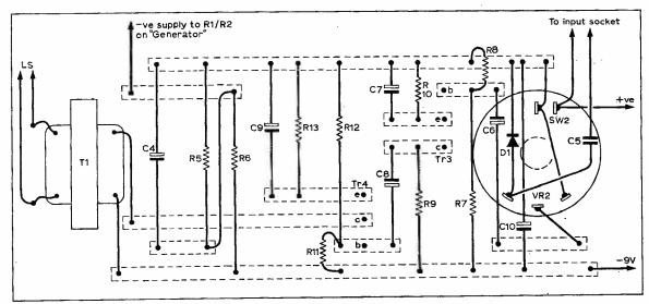
Fig. 3: Layout of the "tracer" circuit board, also full scale
