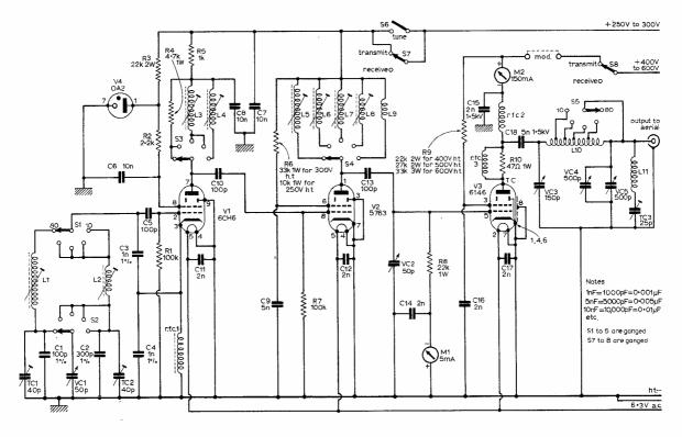
Fig. 1: Complete circuit diagram of the 5-band transmitter.
