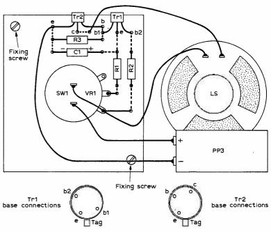
Fig. 2: The component layout and transistor base connections
