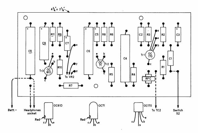
Fig. 2: Top view of circuit board and identification of transistor connections.
