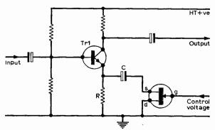
Fig. 4: The basic control circuit used in the final circuit.
