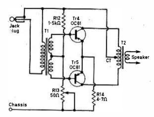
Fig. 7: Circuit of amplifier module.
