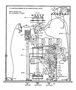
Fig. 3: Underneath the chassis showing main wiring.
