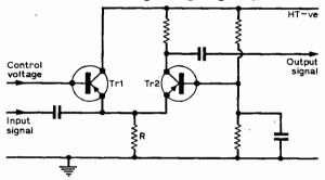
Fig. 3: Two transistors connected as a long tailed pair can control dynamic range but only at low input levels.
