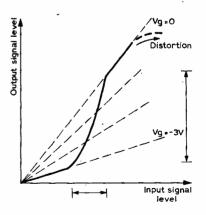
Fig. 8: (left) Expansion circuit principle. Fig. 9: (above) The arrows on the graph show how a small range of volume in the input is expanded to a wider range.
