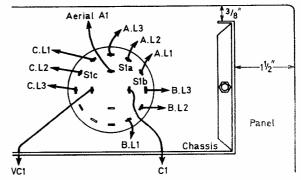
Fig. 6: Position of chassis relative to panel and bandswitch connections
