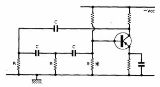
Fig. 5.3. Typical oscillator circuit utilising a CR feedback network
