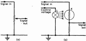
Fig. 1: A standard volume control and a simple method of audio expansion or compression using an L.D.R.
