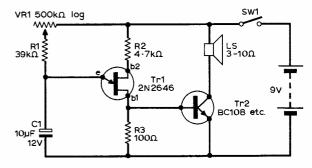
Fig. 1: The circuit of the metronome
