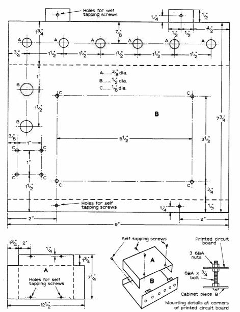
Fig. 12: The cutting and drilling details of the two piece aluminium cabinet.
