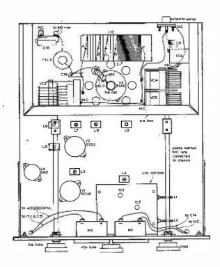
Fig. 2: Plan view of transmitter chassis.
