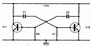
Fig. 5.6. Relaxation oscillator using two feedback networks C1R1 and C2R2
