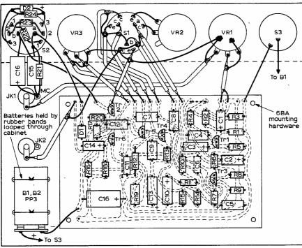
Fig. 11: The component layout. Using the recommended P.C. board makes for easy construction and a neat final layout.
