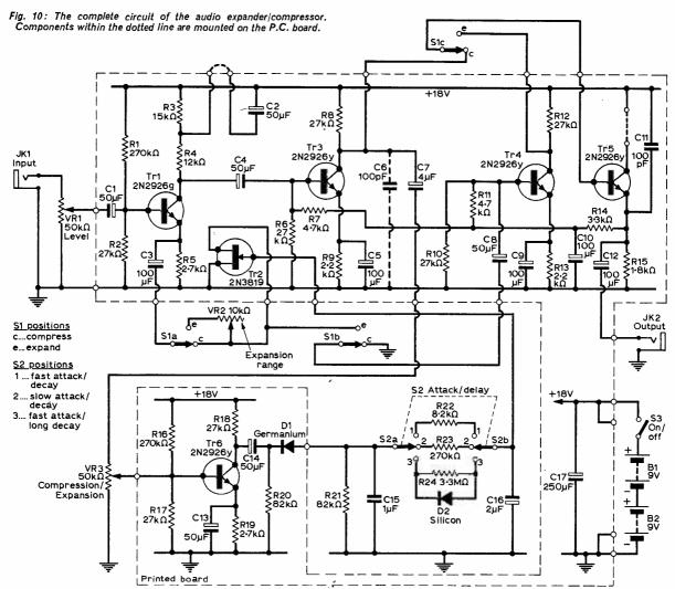
is amplified by Tr3 and fed via C7 and VR3 to Tr6 which is the amplifier A in Fig. 4. The degree of compression (or expansion) is controlled by VR3. The signal at Tr6 collector is rectified by D1, smoothed by C15 and fed to the f.e.t. gate via one of the sets of time constant components selected by S2
