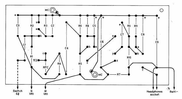
Fig. 3: Bottom view of circuit board showing interconnection of components.
