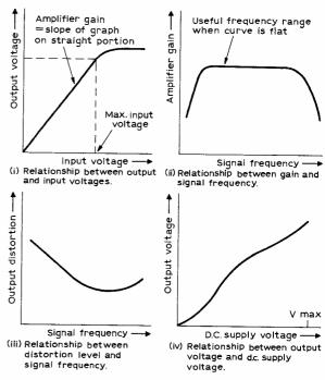
Fig. 2.3: Examples of graphs showing amplifier characteristics
