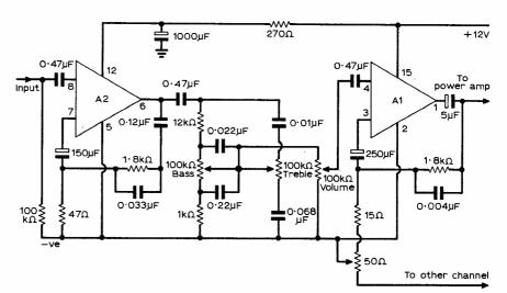
Fig. 2: Circuit for a tone control unit utilising two of the amplifiers for one channel of a stereo preamplifier.
