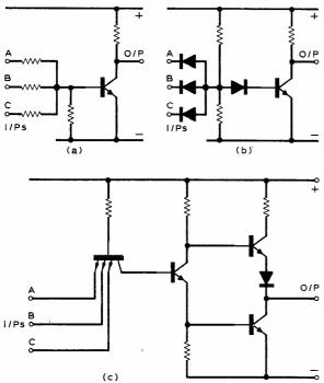
Fig. 12: Three typical logic systems.
