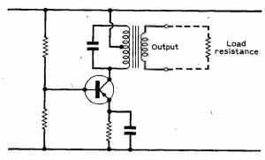
Fig. 2.6: Typical tuned amplifier stage
