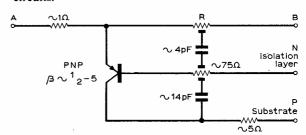
Fig. 11: Parasitic elements of diffused resistor structure.
