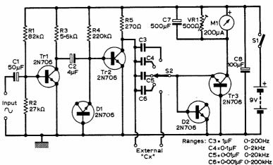
Fig. 2: Circuit of the Frequency Meter
