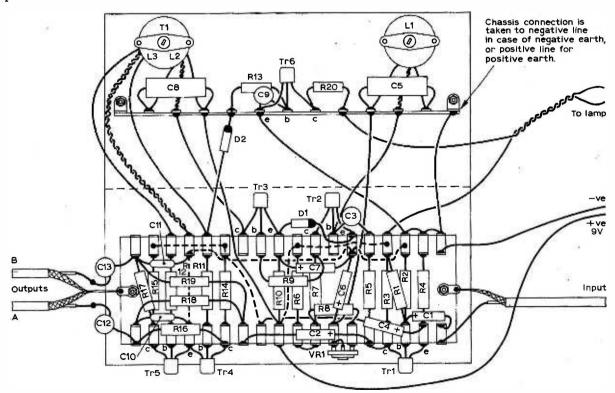
Fig. 4: Component layout and wiring details.
