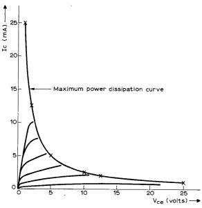
Fig. 2.2: Plot of maximum power dissipation
