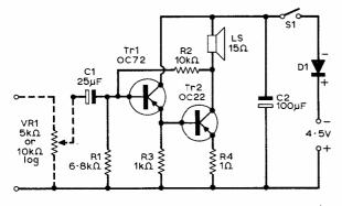
Fig. 1: Circuit of amplifier
