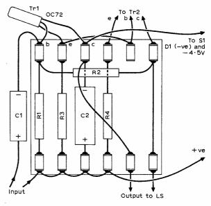
Fig. 3: Component board
