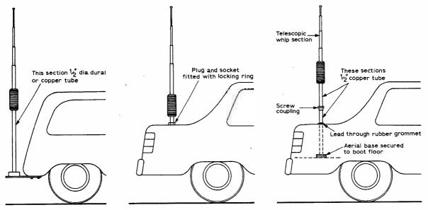
Fig. 7:8:9: Three possible methods of mounting whip aerials
