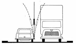
Fig. 6: Importance of adequate rigidity in aerial mountings.
