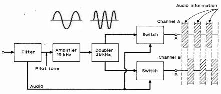
Fig. 1: Block diagram showing operation of decoder
