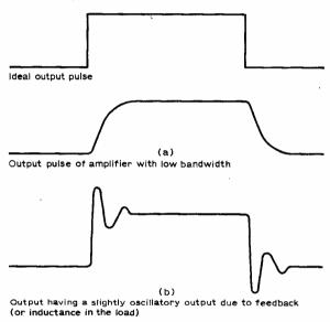
Fig. 2.5: Pulse testing
