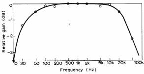
Fig. 2: Response curve of amplifier
