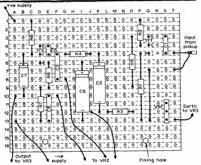
EADERS building the Practical Wireless Pedal Steel Guitar described in the November, December (1969) and January (1970) issues may prefer to assemble the preamplifier on Veroboard rather than plain pin-board, which makes for a tidier layout and some simplification of construc-tion. A prototype Veroboard preamplifier has been built and the layout is given in the accompanying diagram.
