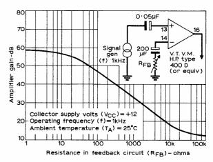
Fig. 6 : Graph showing variation of gain with change in feedback resistance.
