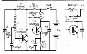
Fig. 1: The circuit of the two transistor radio. If the jack socket is connected as shown a switch is unnecessary.
