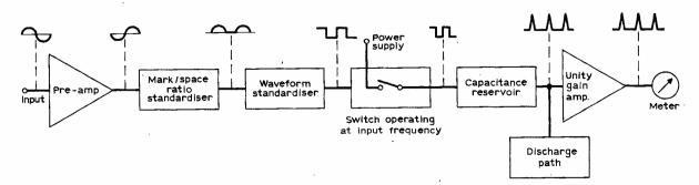
Fig. 1: Block diagram showing stages of the Frequency Meler
