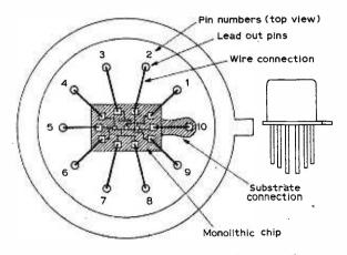
Fig. 15: TO-5 encapsulation and typical chip interconnections.
