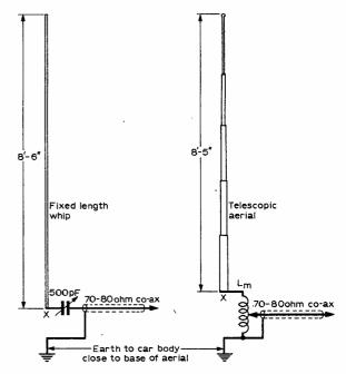
Fig. 4: (Left) Capacity tuned aerial for the 10 metre band.
