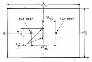
Fig. 4: Mounting board for power transistor
