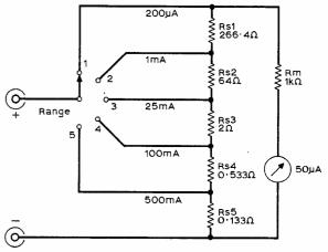
Fig. 8 Final circuit using Universal shunt.
