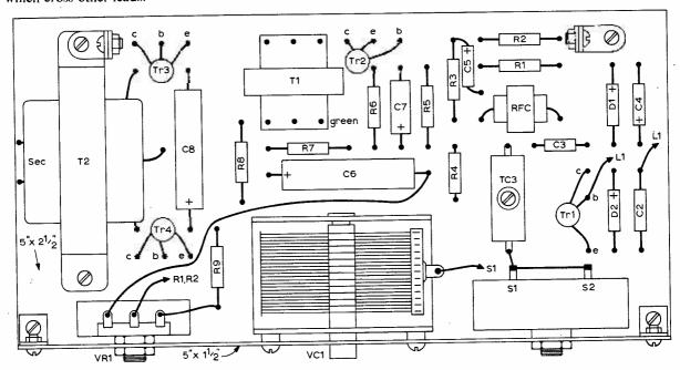
Fig. 2: Top of circuit board with panel attached
