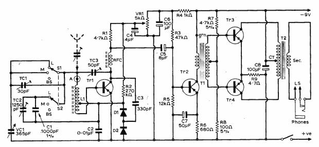
Fig. 1: Circuit of complete receiver
