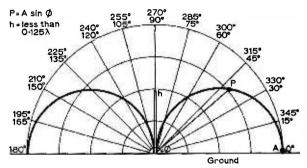
Fig. 1: Radiation pattern of a short vertical aerial.
