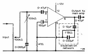
Fig. 3: One channel of a four channel mixer.
