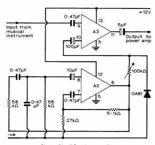
Fig. 4: Circuit for a tremolo unit.
