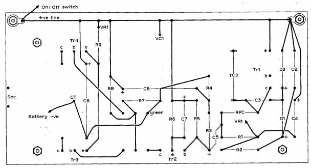
Fig. 3: Reverse side of circuit board
