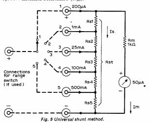
Firstly, to derive a simple formula which will then be used to determine the individual sections of the universal shunt, consider the meter circuit for the lowest current range (range 1). This range uses the total value of the shunt (R<sub>st</sub>), and the simplified circuit looks like that shown in Fig. 6. 'It' is the total current flowing in the testmeter; Is is the current in the shunt, and Im is the current in the meter. Determine the value of R<sub>st</sub> by
