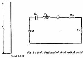
Fig. 3 : (Above) Equivalent circuit of loaded vertical aerial
