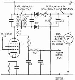
Fig. 17—The basic circuit of a ratio detector, showing the load across which a direct voltage is developed due to the I.F. signals being rectified by the seriesconnected diodes. CI is the A.F. load, RI a currentlimiting resistor, and R2 and C2 the de-emphasis network. The pre-set resistor R4 facilitates a balance adjustment for optimum A.M. limiting.
