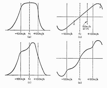
balanced, the detector response would be something like the curve in Fig. 19(b). This would handle full modulation over the linear part of the curve as long as the undeviated carrier were kept fairly close to the centre of the linear part (at point fc). A small deviation from this centre, however, would cause the signal to enter the curved part of the response and result in severe distortion.
