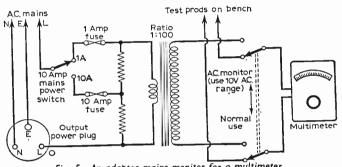
Fig. 5-An adaptor mains-monitor for a multimeter.
