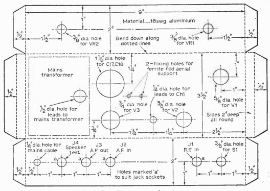
Fig. 3—The drilling dimensions of the chassis.
