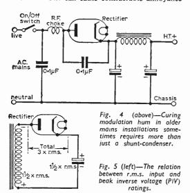
to one's neighbours with an unsuitable rectifier circuit, as well as impair the performance of one's own equipment. Notorious offenders are A.C./D.C. sets drawing H.T. through a rectifier connected direct to the mains, as this arrangement offers easy entry and exit of R.F. signals over the mains. Sets using a transformer are far better, and in many cases the R.F. losses of the mains transformer are high enough to remove all trace of modulation hum even without rectifier-shunt condensers.
