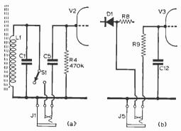
Fig. 2a—A modification of the circuit, omitting VI; b—An additional input to the grid of V3.
