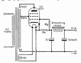
Fig. 2—Feeding the screen from a tap on the transformer instead of strapping it to the anode.
