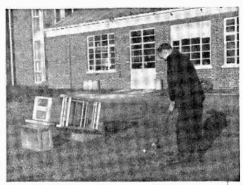
The Marconi Sea-EVA (Electronic Velocity Analyser), was experimentally demonstrated recently to a technical representative of the Dunlop Sports Co. Ltd. as being suitable for gathering data on golf balls.
