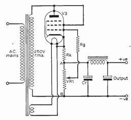
Fig. 3—A variable output circuit using an EL34.
