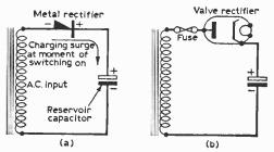
Fig. 1a—A fuse taken direct from the transformer to the rectifier would be likely to blow easily on switching on, due to the charging surge of the reservoir condenser;
