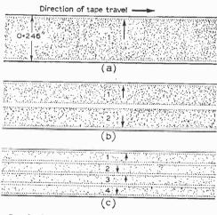
Fig. 9—Recording tracks and directions: (a) single track recording, (b) two-track recording and (c) four-track recording. (The arrows on the tracks indicate the top of each track during the recording process.)
