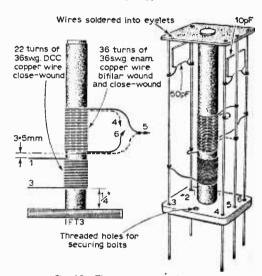
Fig. 10-The construction of IFT3.
