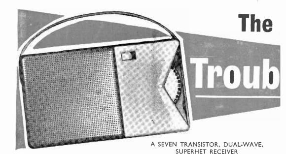
HIS receiver uses seven transistors in a superhet circuit, and will be found to give very good results indeed, with ample volume in even unfavourable circumstances. It tunes both medium and long waves and fits in a ready-made cabinet which is approximately  $5\frac{1}{4}$  in.  $\times 3\frac{1}{8}$  in.  $\times 2$  in. (external dimensions). It is thus very compact and portable, and is capable of a really good output from the internal speaker.
