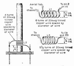
Fig. 8-The construction of L1, L2, and L3.
