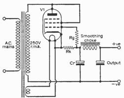
Fig. I—Using the normal cathode bias and grid leak resistors with an output valve as rectifier.
