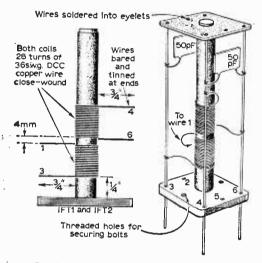
Fig. 9-The winding data for IFTI and IFT2.
