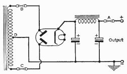
Fig. 2 (above)—Possible positions for fuses in a fullwave rectifier circuit.
