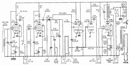
Fig. 1-The circuit of the instrument.
