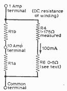
current-carrying capacity must be considered when replacing the experimental shunt by separate final shunts between the input terminals of the various ranges. Each sub-shunt must capable of carrying the current represented by the input terminal to which it is connected on the side away from the common terminal. Any length of wire, as shunt between two terminals, which is to be capable of
