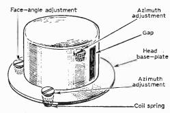
Fig. 12—One arrangement used for the face-angle adjustment and the azimuth adjustment of the record/replay head.
