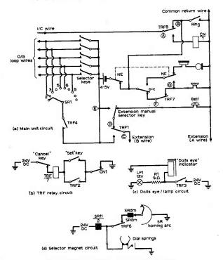
Fig. 9: Wiring of the auto-transfer facility.
