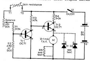
Fig. 1: The lie detector circuit. D1, D2 and R5 are meter protection components.
