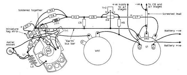
Fig. 2: Layout of the tuner section of the receiver. The audio amplifier stages are not shown. C3 may alternatively be of the "twisted wire" variety (see text). The leads of L2 should be kept as short as possible, one end being soldered directly to the fixed plate of VC1 (5pF type C804 shown in the above diagram).
