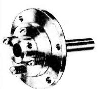
The adjustable-torque ball-drive with reduction ratio of 6:1. The spring-loaded screws to the left of the photograph effect the adjustment of the torque.
