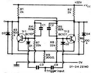
Fig. 4.4: The counter of Fig. 4.3 requires two supply rails. By lifting the bases above ground with R9 in this circuit, only one supply is required.
