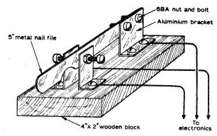
Fig. 2: The keyer paddle mounted on a wood block.
