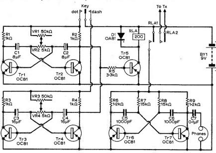
Fig. 1: The complete circuit of the electronic keyer.
