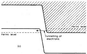
Fig. 4: (a) Tunnel diode energy band diagram when in an open circuit state of equilibrium. (b) Tunnel diode with reverse bias, (c) with small forward bias.
