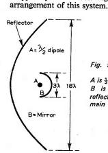
Fig. 5.10: A parabolic dish aerial for s.h.f.
