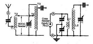
Fig. 5.3: A transmitter output impedance match for balanced
