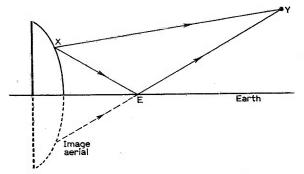
Fig. 5.5: How the image of an aerial affects its radiating properties.
