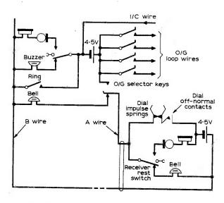
Fig. 6: Wiring of the two-wire connected extension.
