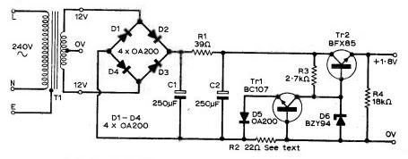
Fig. 2: The circuit of the power supply.
