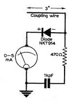
The general constructional details are left to the constructor. The few components used may be grouped at the back of the meter on a piece of Veroboard and the assembly then mounted in a suitable wood or metal box.
