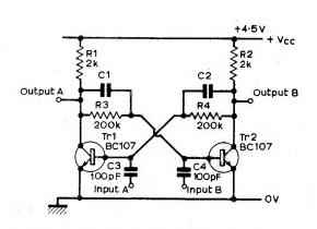
Fig. 4.1: The simplest form of bistable circuit, which rests in either of two stable states, changing only on application of trigger pulses. C1 and C2 are speed-up capacitors for improving switching times.
