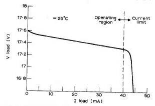
Fig. 1: Typical output voltage plotted against load current.
