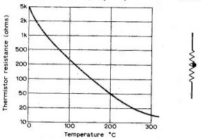
Fig. 3 (right): Thermistor circuit symbol. Fig. 4 (left): Thermistor logarithmic characteristic,
