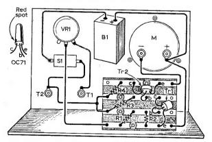
Fig. 2: Wiring of the lie detector and transistor lead identification.
