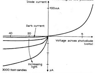
Fig. 3: Photodiode characteristic curve showing change in reverse current with change of light intensity.
