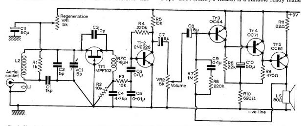
Fig. 1: Circuit of the complete receiver. If only the tuner is required (as depicted in Fig. 2), the audio output should be taken from the slider of VR2. S1 should be shown wired in the +9V supply lead.
