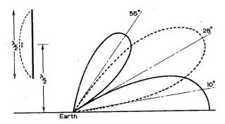
Fig. 5.7(a): The radiation patterns from a  $\lambda/2$  aerial  $\lambda/2$  above ground.
