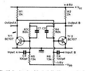
Fig. 4.2: An adaptation of the simple bistable to ensure that the non-conducting transistor is completely cut-off.
