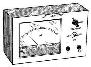
Fig. 3: Appearance of the instrument.
