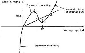
Fig. 5: Tunnel diode characteristic curve.
