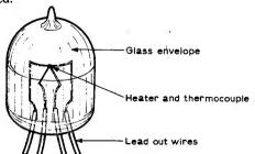
Fig. 7: Vacuum v.h.f. thermocouple.
