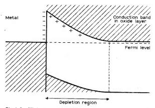
Fig.1: Equilibrium energy band diagram for a metal-oxide rectifier.
