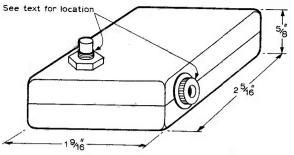
Fig. 4: The plastic case for the Mini-two.
