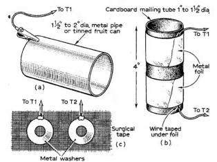
Fig. 4: Skin resistance electrodes; (a) for holding in each hand, (b) for holding in one hand and (c) for taping to wrist.
