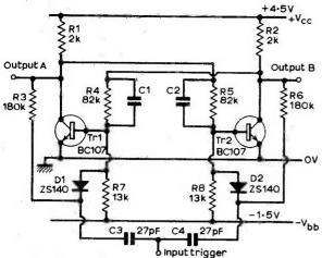
Fig. 4.3: The bistable can be usefully employed in counters, by modifying the circuit as shown here. The input pulses are divided sequentially by the steering circuit consisting of D1/2, R3/6, C3 and C4.
