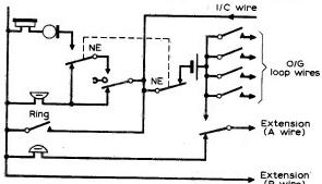
Fig. 8: Wiring of the two-wire night extension.
