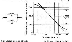
Fig. 5: Linearising the thermistor characteristic.
