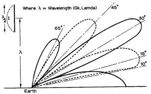
Fig. 5.7 (b): The λ/2 aerial one wavelength above ground produces a much more satisfactory pattern.
