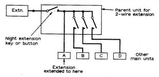
Fig. 7: Block diagram of two-wire night extension.
