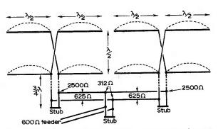
Fig. 5.8: The Koomans multi-element aerial array produces a much more predictable pattern than single  $\lambda/2$  aerials.
