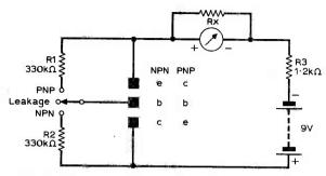
Circuit of the tester. See text for details on meter and Rx.
