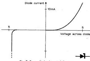
Fig. 2: Zener diode characteristic curve.
