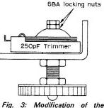
Fig. 3: Modification of th tuning trimmer.
