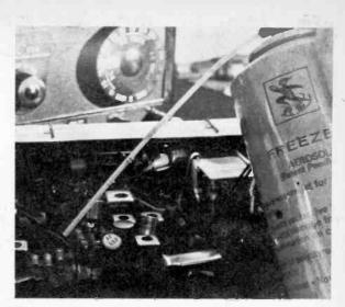
A quick test for noisy components is a squirt of freezer from an aerosol.
