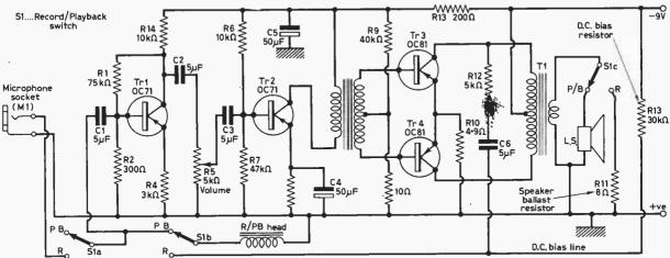
Fig. 8: A practical transistor tape recorder amplifier.
