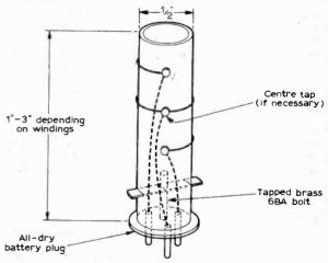
Fig. 11: The Author's method of coil construction.
