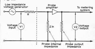
Fig. 5: Measuring the input impedance of the probe.
