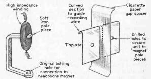
Fig. 1: The headphone electromagnet.
