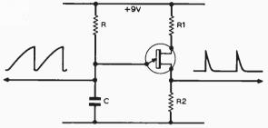
Fig. 18: Simple unijunction oscillator circuit.
