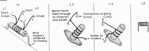
5+5 turns, 32s.w.g. enamelled, bifilar wound in groove of RS type A core.
