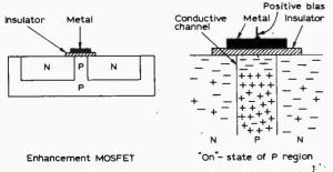
Fig. 16: Principle of the enhancement-mode insulated-date field effect transistor (m.o.s.f.e.t.).
