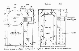
Fig. 7; Details of the aluminium case.
