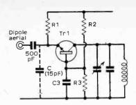
Fig. 2: An alternative untuned input circuit.
