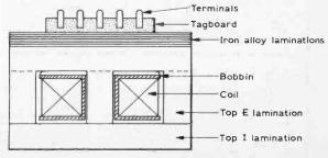
Fig. 4: Basic coil construction.
