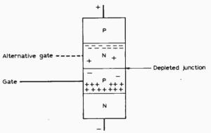
Fig. 17: The thyristor is a four-layer device with three pn junctions.
