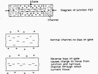
Fig. 15: Principle of the junction-gate field effect transistor.
