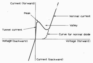
Fig. 14: Tunnel diode current-voltage characteristic.
