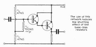
Fig. 2: A modification to Fig. 1a which reduces the shunting of the bias resistors.
