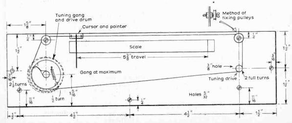
Fig. 4: Layout of the front panel, seen from the rear, with assembly details for the cord dial drive.
