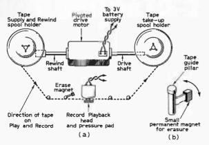
Fig. 7: The tape transport and erase systems.
