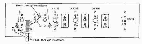
drilled through the paxolin centres showing through the holes previously drilled in the chassis, and through which the transistor leads will be inserted later.
