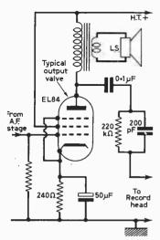
Fig. 3: Tapping off from an output valve.
