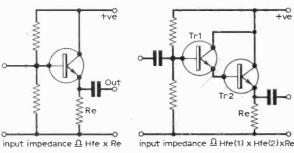
Fig. 1: A conventional emitter-follower and (a) a compound version with a higher input impedance.
