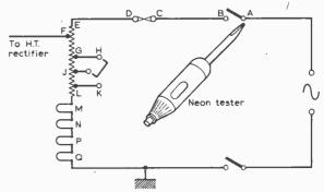
Fig. 2: The ubiquitous neon tester is useful for rapid continuity tests of AC/DC receivers, with the power applied in the correct polarity.
