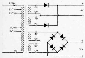
Fig. 7: Multi-turn transformer with rectifiers.
