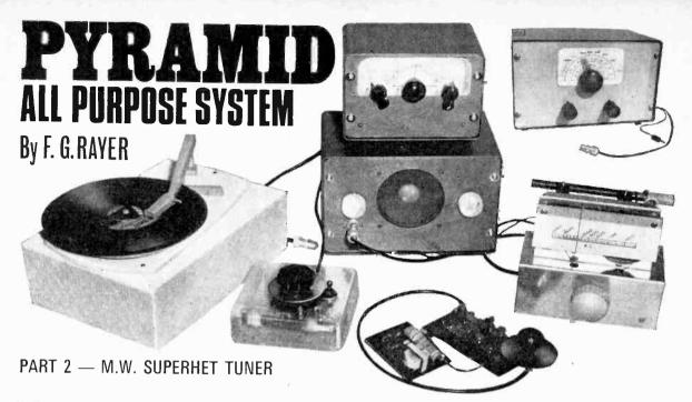
THIS tuner is primarily designed for plugging into the "Pyramid" amplifier, for immediate reception over the medium wave band. Long wave coverage can be added later, if wanted. The tuner could be used with other amplifiers, or for excellent phone reception, for personal listening.
