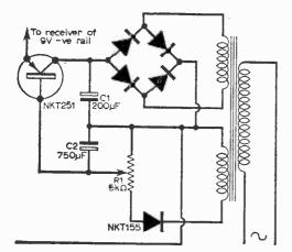
Fig. 5: Stabilised power supply circuit for battery/mains transistor sets (Ferranti). The entire d.c. output passes through the NKT251 power transistor to the receiver's negative rail. Variations in mains voltage produce similar variations across RI which are applied to the base of the transistor so that its internal resistance is varied accordingly. When mains voltage rises its internal resistance increases, taking up a larger volts drop, and maintaining output within very close limits.
