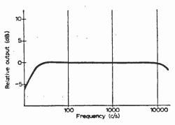
Fig. 17 (a): Playback head curve showing response for signal of constant recording level.
