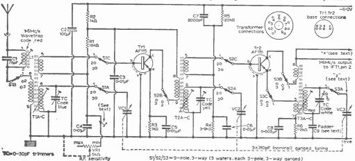
Fig. 1: Complete theoretical circuit diagram of the bandswitched front end. In the interests of clarity only one transformer for each range is shown.
