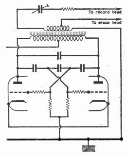
Fig. 15: Push-pull r.f. oscillator to minimise second harmonic distortion.
