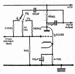
Fig. 18: Playback equalizing circuitry for three speeds.
