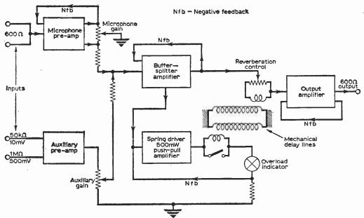
Fig. 16: Schematic diagram of commercial reverberation unit (Grampian 636).
