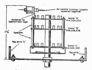
Fig. 4: Switch wafer arrangement and trimmer location.
