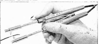
The new ADAMIN thermal wire strippers allow one-handed operation, using a simple tweezer action.
