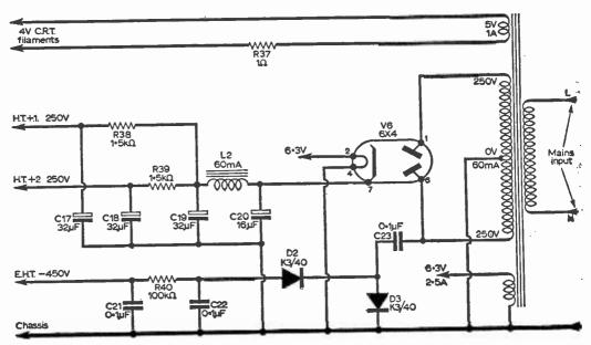
Fig. 4: The oscilloscope power supply unit.
