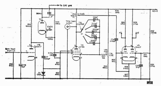
Fig. 2: The timebase and symmetrical deflection amplifier (X-amp). The dotted components comprise the flyback blanking
