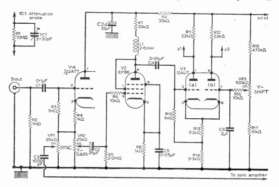
Fig. 1. Vertical amplifier (Y-amp) with symmetrical deflection and probe unit.
