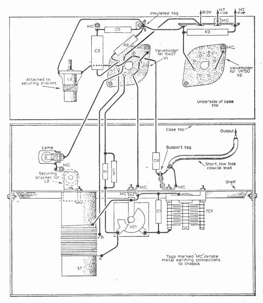
Fig. 2: The complete, ring diagram of the finished unit.
