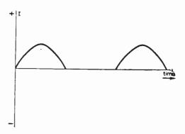
Fig. 47: Current flowing in the anode circuit of a simple diode rectifier.
