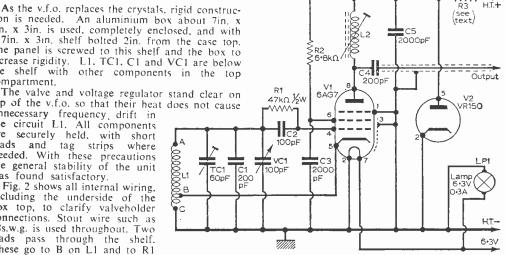
Fig. 1: The v.f.o. circuit. The operation of this simple circuit is described in the text.
