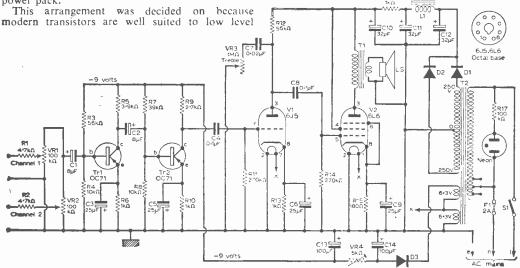
Fig. 1: The basic hybrid circuit of the "Cadet", complete with preamplifier stage and power supply.
