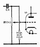
Fig. 2: The modification to the VI circuitry to provide a high level input. This allows for the use of record player, carbon microphone and similar inputs with the amplifier.
