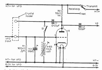
rig. 3: Using VI of the original transmitter circuit (page 855, January issue) as a frequency doubler.
