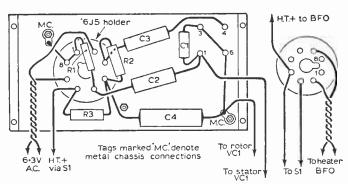
Fig. 9 (above): The position of the b.f.o. unit on the main chassis. The shaded parts indicate components on the original receiver.
