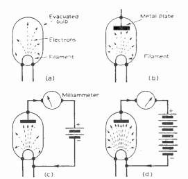
Fig. 38: A heated filament in an evacuated bulb emits electrons (a), some of which strike the metal plate (b). When a positive potential is applied to the plate, more electrons are attracted to it (c) and the greater the potential, the greater the electron flow (d).
