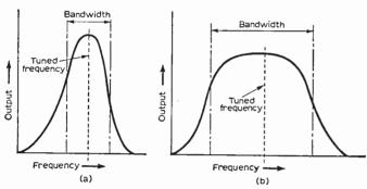
Fig. 4: Response curves. The narrow curve of restricted bandwidth (a) may attenuate the treble response and also aggravate the effects of oscillator drift in f.m. sets, and in f.m. sets the wider response of (b) is often to be preferred. A response of extended bandwidth cannot, however, be used in a.m. sets for fear of adjacent stations breaking into the wanted tuned station.
