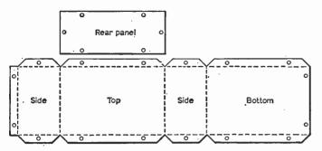
Fig. 8 (above): Another method of constructing a cabinet on the lines of that of Fig. 7, and Fig. 9 (below): an easier method of achieving the same result.
