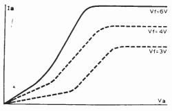
Fig. 44: Characteristic curves using different heater voltages.
