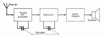
Fig. 1: Block diagram of tuned radio-frequency receiver.
