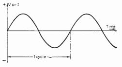
Fig. 46: Typical a.c. waveform.
