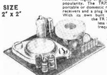
Another highly original Sinclair design which enjoys enormous popularity. The TR750 amplifier makes a powerful car, portable or domestic radio used with the Micro-6 or Slimline receivers and a plug is included for connecting to these sets. With its own built in volume control and on-off switch, the TR 750 has a full 750 milliwate transformer-
