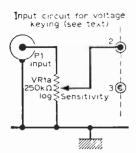
Fig. 2: The P1 input of the circuit of Fig. 1 modified for voltage keying.
