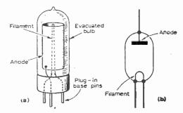
Fig. 39: The diode: (a) practical representation;
