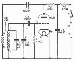
Fig. 7: The one-valve circuit of the b.f.o. unit.
