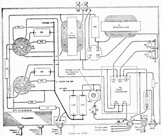
Fig. 4: Complete wiring details of the main amplifier and power pack chassis.
