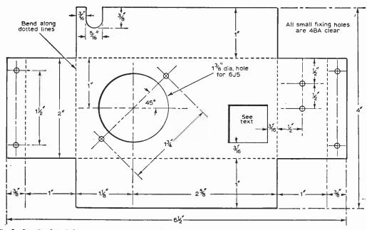
Fig. 8: Details of the b.f.o. chassis which is eventually attached to the main receiver chassis. This arrangement may be seen in one of the heading photographs on page 1055.
