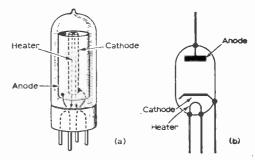
Fig. 40: The indirectly heated diode, practical construction (a) and theoretical representation (b).
