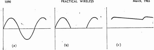
Fig. 49: The a.c. waveform: (a) before rectification; (b) after rectification and (c) with smoothing capacitor.
