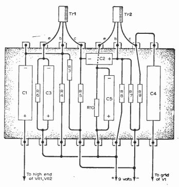
The 250V supply is smoothed Fig. 5: Construction details of the preamplifier chassis which is built separately and fitted to the underside of the main chassis when complete.
