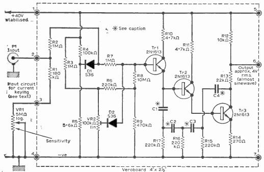
Fig. 1: The oscillator circuit. The output frequency is determined by the capacity of the four (equal) capacitors C1-C4.
