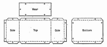
The cabinet of Fig. 7 is very robust but difficult to bend. The same final shape can be obtained by using a number of different methods of construction, as shown in Figs. 8 and 9.
