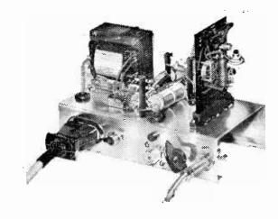
(small paxolin sheet with regular rows of holes for affixing components, as described in PRACTICAL WIRELESS, May 1964) and has seven terminals for external connections (Fig. 1).
