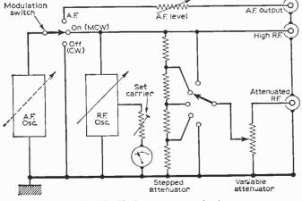
Fig. 18: The basic generator circuit.
