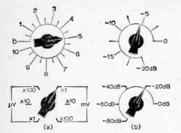
Fig. 20: Two examples of attenuator control markings.
