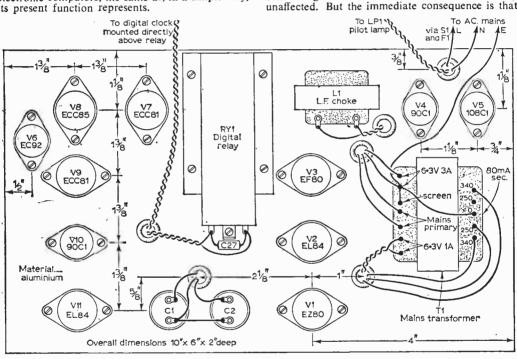
Fig. 3: Above-chassis layout and wiring, showing main drilling dimensions.
