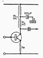
Fig. I: A method of reducing the voltage developed across the collector on signal by using a large by-pass capacitor across the greater part of the load.
