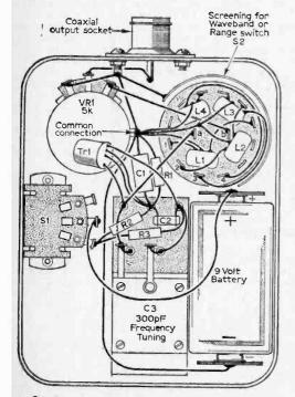
Fig. 2: Interior view showing layout and wiring.
