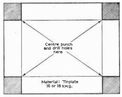
Fig. 1: Cutting the chassis.
