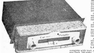
Battery drain is exceptionally low—the life of the self-contained battery within the set is approx. 200 hrs. Transistors used: 1 OC44: 2 OC45: 1 OC4201; 2 OC82 and Diode. Compares with set costing at least double, properly installed this set will give you years of pleasure and service both in and out of your car.
