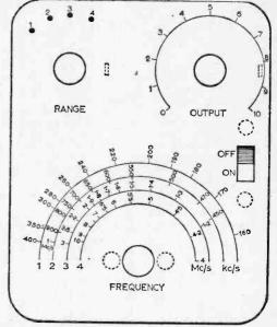
Fig. 3: Oscillator scale plate. This is made up from 18s.w.g. aluminium covered with drawing paper.
