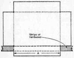
Fig. 2: Bending the cut tin plate
