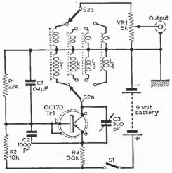
Fig. 1: Circuit diagram of the oscillator.
