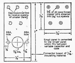
Fig. 5: Connector board, made up of  $\frac{1}{16}$  in. insulating material.
