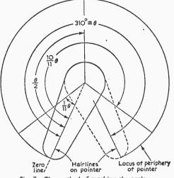
Fig. 7-The method of marking the scale.
