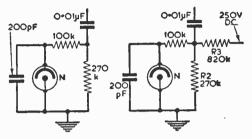
Fig. 3—A simple indicator circuit using a neon. Fig. 4—A neon indicator circuit with bias.
