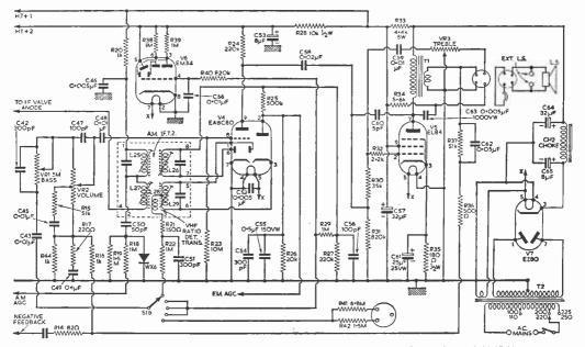
Fig. 9-The circuit diagram of the detector, AGC, A.F., output and rectifier stages of a combined A.M./F.M. receiver.
