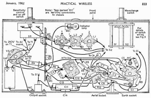
Fig. 2b—The under-chassis layout and wiring diagram.
