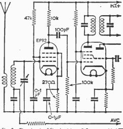
Fig. 2-The circuit of Fig. I with an R.F. stage added.
