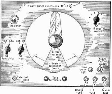
Fig. 5-The layout of the front panel.
