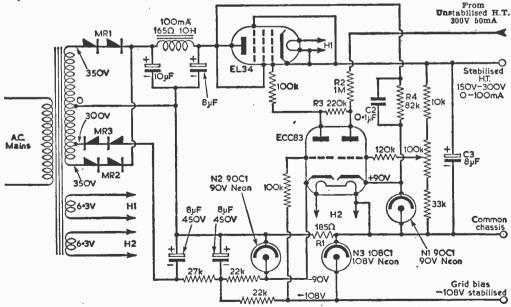
Fig. 3-The advanced stabilising circuit with the addition of an effective current limiting circuit.
