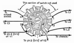
Fig. 3—Utilising a 3-pole, 4-way, rotary switch for band selection.
