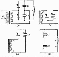
Fig. 14 (a)—The complete voltage doubler circuit. (b)—When the supply voltage is as shown in the diagram, C2 is charged.
