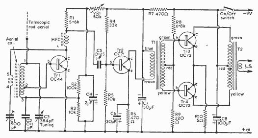
Fig. 1-The circuit of the receiver.
