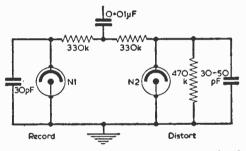
Fig. 5—A circuit using two neons; one for record and one for over-record.
