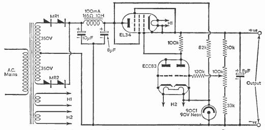
Fig. 1—The basic stabilising circuit without any form of current limiting device.
