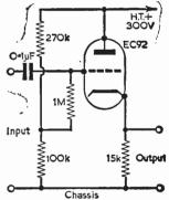
Fig. 6—A cathode-follower circuit, capable of handling peak 75V signals (positive or negative).
