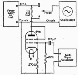
Fig. 5—Method of measuring dynamic internal impedance.
