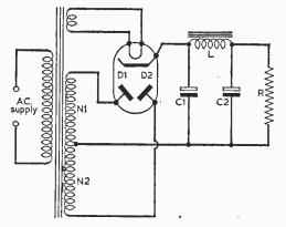
Fig. 9-A complete H.T. full-wave rectifier circuit.
