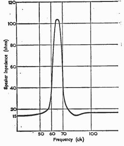
Fig. 1—A typical resonance curve for a  $15\Omega$  speaker with a 65c/s resonance.
