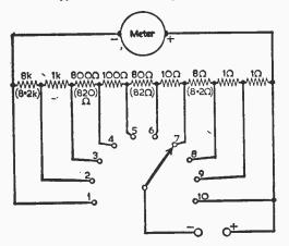
Fig. I—A circuit of a switched universal shunt. The figures in brackets are preferred values of components which may be used if extreme accuracy is not essential.
