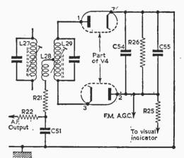
Fig. 10—The ratio detector section from the receiver shown in Fig. 9 with the same component references.
