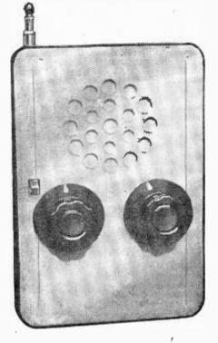
HE TRF type of receiver is much easier to construct than a superhet, and does not require any form of trimming or alignment whatsoever. It is thus particularly suitable for use when a straightforward circuit giving reception of local stations only is required. The circuit shown in Fig. 1 has four transistors, and gives very good speaker results, in these circumstances.
