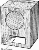
Fig. 2-A bass reflex cabinet showing the rectangular vent and tunnel beneath the speaker.
