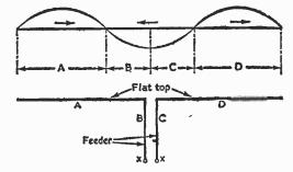
to the feeder ends X. A static impulse will, however, flow down B and C in the same direction, and thus cancel out at the tuning coil. This explains the reduction in static interference. Cancellation will not in fact be complete, owing to lack of exact balance, but will usually be worthwhile.
