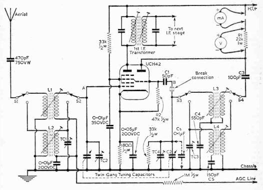
Fig. 1.—The local oscillator or frequency changer stage of a superhet receiver.
