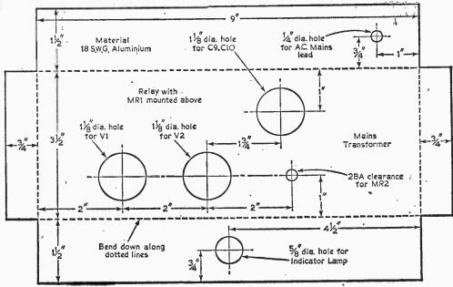
Fig. 2.—The drilling dimensions of the aluminium chassis.
