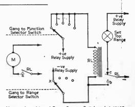
Note: x is position of Range Selector Switch on top range
