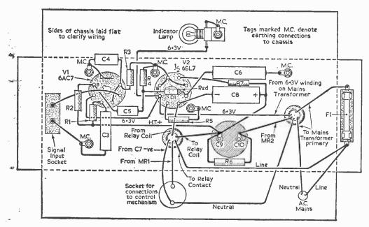
Fig. 3.—The underchassis wiring diagram.
