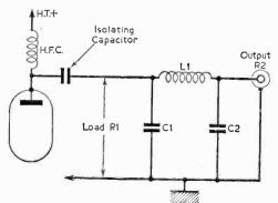
Fig. I (above).—A typical  $\pi$ -network output circuit.
