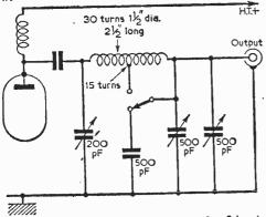
Fig. 3.—A π-network output circuit for 2-band operation.
