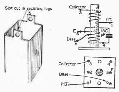
Fig. 5.—The mounting lugs of the transformers are cut as shown to enable them to be passed over the fixing bolts (see text).
