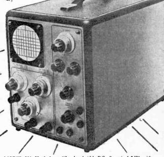
MODEL 381. Vertical amplifier bandwidth DC—9 mc/s (-3dB) with rise time of .06  $\mu$ Sec., and overshoot of less than 1%. Calibrated nine stage frequency compensated input attenuator. In addition all the facilities of a high class 3" general purpose oscilloscope. Unique mechanical construction with all panels removable for ease of maintenance. Convection cooled.
