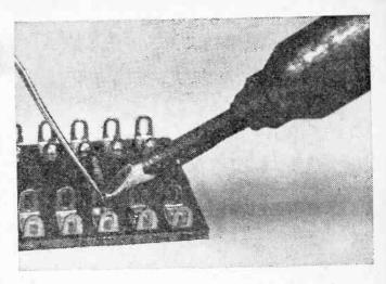
(Above) Soldering a resistor to a tag-board, and (below) using pliers as a heat shunt when soldering transjstor leads.
