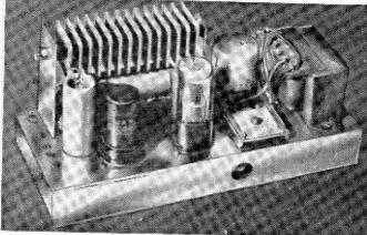
HIS apparatus was designed so that the door of a garage could be made to open automatically on receipt of a command signal from the driver of an approaching vehicle. It is, of course, suitable for any other control service where only a short range is required. While the mechanical part of the installation is rather outside the scope of these pages, it must be said briefly in explanation that the controlled door is of the roller shutter type which, when the retaining bolt is withdrawn, rises
