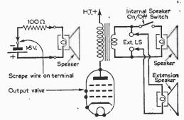
Fig. 2 (left).—A method of checking loudspeakers. Fig. 3 (right).—Here, an extension speaker is used and an on/off switch is incorporated in the circuit.
