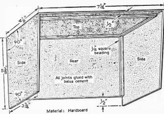
Fig. 1.—The dimensions of a suitable cabinet for any of the receivers.
