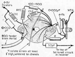
Fig. 3.—The layout of the R.F. preamplifier.
