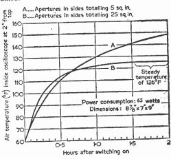
Fig. 1.—The curve "A" represents the result of inadequate ventilation, curve "B" with more ventilation.
