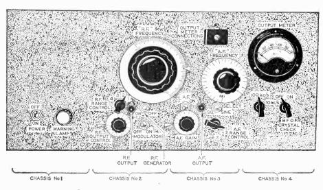
Fig. 36.—The front panel of the completed signal generator.
