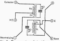
Fig. 7.—The connections of the I.F. transformer windings.
