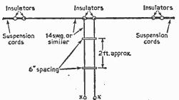
A balanced aerial can also give a considerable reduction in static and similar noise, compared with a single wire or end-fed or end-coupled aerial. This reduction in noise is somewhat similar to that achieved with a coaxial feeder.
