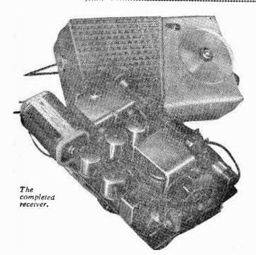
touch the speaker. The speech coil is then wired to the output transformer secondary. This is most readily achieved by soldering short lengths of thin flex to the speech coil tags before mounting the speaker. These may then be soldered to brown and purple tags of the transformer.
