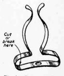
Fig. 2.—Preparing the spring clips.
