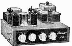
HARMONIC DISTORTION 1.000 than 0.1% measured at 8 watts at 1000 c.p.s. Weight 10 lbs. Power consumption 90 watts. For 200-230-250 v. 50 c.p.s. A.C. mains. Outputs for 3-and 15-ohm speakers. Chassis finish stoved Gold hammer.
