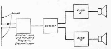
Fig. 1(b).—A decoder unit in the receiver separates the two signals.
