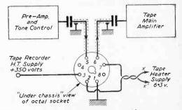
Fig. 5.—Outlet connections for socket on taperecorder.
