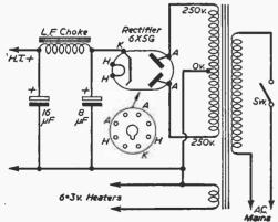
Fig. 5.—Circuit of the power pack.
