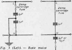
interference suppression circuit. (Note: the condenser between
