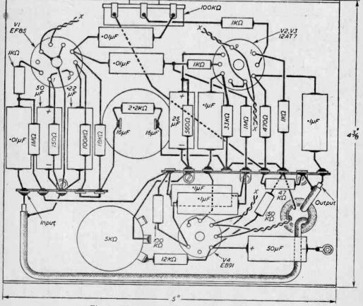
Fig. 6.-The underchassis wiring of the AVC unit.
