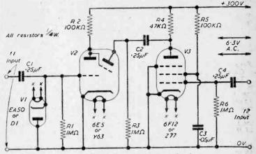
Fig. 4.—Frequency comparator circuit.
