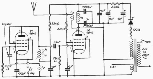
Fig. 1.-Circuit of the transmitter.
