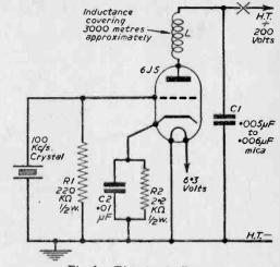
Fig. 1.-The circuit diagram.
