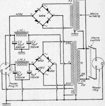
Fig. 7 .- The revised circuit of the power pack.
