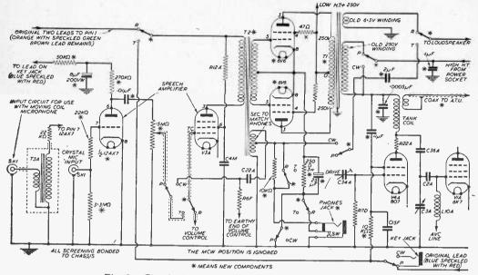
Fig. 8.-Circuit diagram of the transmitter modifications.
