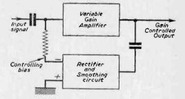
Fig. 1.-Block diagram of the AVC unit.
