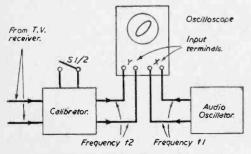
Fig. 2.—Calibration using a cathode ray oscilloscope.
