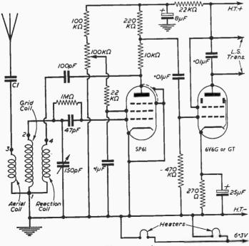
Fig. 1.—The circuit diagram.
