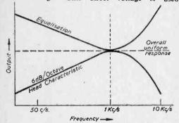
Fig. 2.—Tape playback response showing the effect of equalisation.
