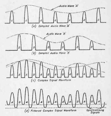
Fig. 4.—Various waveforms at the transmitter (a) and (b). Output waveforms from the encoding mixers. (c) The complex signal obtained two equal linear, symmetrical by adding the outputs from the encoding mixers. (d) A symmetrical and independent signal paths waveform obtained by adding a small amplitude component at the and therefore is capable of sampling or multiplexing frequency in phase quadrature with both sampling pulse trains.
