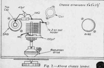
between heater pins as this type of valve will not fit international octal holders. The various "M.C." connections go to tags bolted to the chassis. Coloured flex can be used to identify the various external connections. All leads in the set are shown in Figs. 2, and 3, and these layouts should be followed fairly closely.
