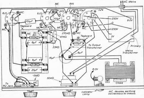
Fig. 3.—Wiring beneath the chassis.
