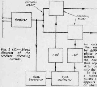
At the receiver, standard components up to and including the frequency discriminator are used followed by a decoding apparatus and two conventional audio stages. (See Fig. 1(b).)
