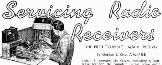
HE Pilot "Clipper" is a table model having a V.H.F.-F.M. band in addition to the M.W. and L.W. bands. It features a built-in compressed dipole for V.H.F., an internal ferrite rod aerial for the A.M. bands, a reduction drive to facilitate accurate tuning and a full length illuminated station scale. There is also a large loudspeaker which is
