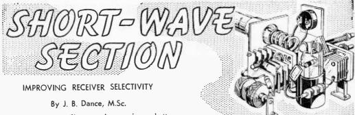
THE short-wave listener who requires a better performance from his receiver must adopt some method of obtaining increased selectivity. The two methods most frequently employed are the use of crystal filters and conversion to a double superheterodyne.
