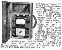
The Weston Model 772 Type 6 super sensitive analyser. This preanalyser. This pre-cision designed multi-range test instrument has a large visible finely divided scale giving some of the range shown. Range D.C. volts 20.00 ohms per volt of 20.000
