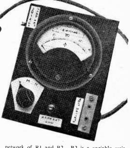
network of R1 and R2. R2 is a variable resistance. and is called the set-zero control, its function is to maintain FSD even when the torch cell voltage falls off with use. The overall value of the required series resistance is given by Ohm's Law, which may be written mathematically as R = V/I, where R is the resistance in ohms. V the applied voltage, and I the current in amperes. In this particular case the FSD current is 4 milliamperes, i.e. 4/1.000 ampere, and the applied voltage is 1½.
