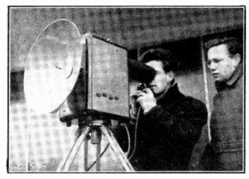
The Tellurometer master instrument being operated by a trainee, seen here receiving instruction.
