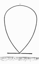
Fig. 5.—The effect of ground reflections on an aerial close to the ground is to concentrate energy skywards. This situation applies especially in topband and eighty metre working.
