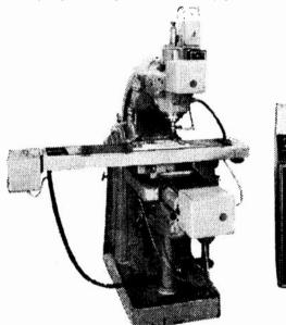
A standard vertical milling machine equipped with a complete three-dimensional control system, using magnetic tape.
