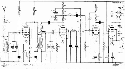
Fig. 1. Theoretical circuit of the Mains T.R.F. Short Waver,
