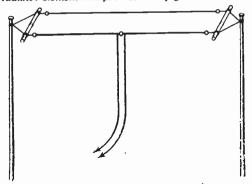
Fig. 9.-A "Flop-over" wire element beam supported on bamboo spreaders.
