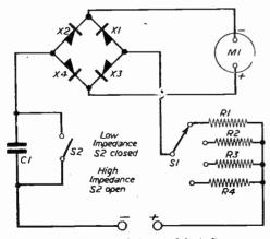
Fig. 1.—Theoretical circuit of the indicator.
