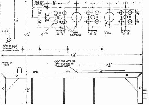
Fig. 3.- Details of the chassis and drilling.
