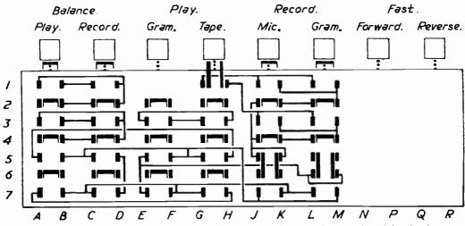
Fig. 4. - Press-button unit with buttons in " off" positions. View from bottom of amplifier chassis.
