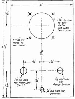
Fig. 4 .-- Details of the panel.
