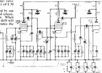
Fig. 1.- Circuit of the R.F.27 unit. Components marked \* are omitted from modified circuit.
