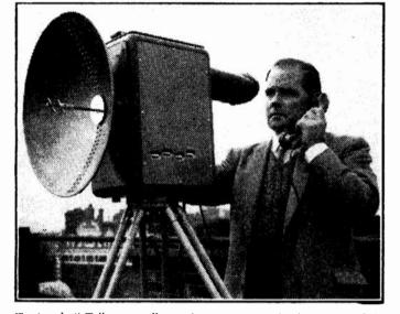
Texting the " Tellurometer "----a micro-wave measuring instrument. It is claimed that this has an accuracy of 2in. to 6in, over distances ranging from 10 to 30 miles,
