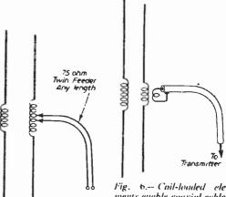
Fig. 5.- Compact coil loaded dipoles may be fed by topping the feeder into the centre of the loading coil. Fig. 6.-- Coil-loaded elements enable coaxial cables to be matched in by a small, tightly coupled link winding wound over the loading coil, a very efficient and hondy method of feeding "Compacted dipole" elements,
