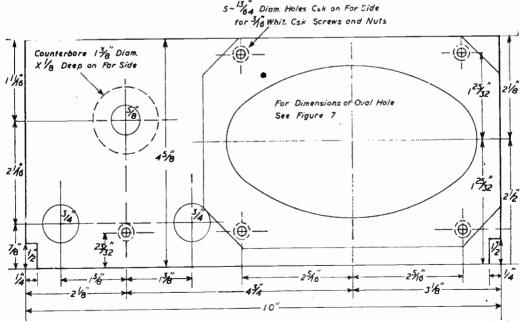
Fig. 4.—Details of the plywood panel, \$in. thick, viewed from rear. Shaped area to be cut away to depth of 1 ply.
