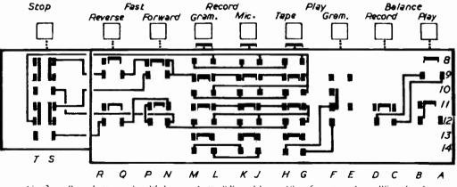
Fig. 3. – Press-button unit with buttons in " off" positions. View from top of amplifier chassis,
