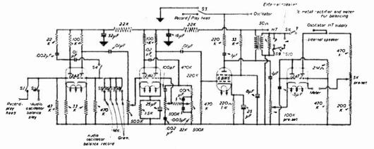
Fig. 1.— Simplified circuit of one amplifier – andio oscillator and rectifier for baloncing signal omitted for simplicity. See also table at foot of next page.
