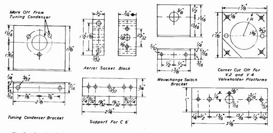
Fig. 8.—Details of the various brackets and other metal fitments.
