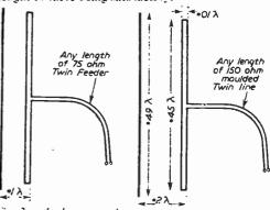
Fig. 3.-- A close-spaced array may have the radiator folded to match 75 ohms line,
