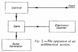
The average pulse generator is generally a multivibrator circuit, although in small machines a squegging type oscillator is often used. An amplifier is also required to ensure a pulse of sufficient amplitude is transmitted. Pulses are produced at a rate of about 100,000 per second. (Different makes and types, of course, vary.) These pulses are routed by gates. If a
