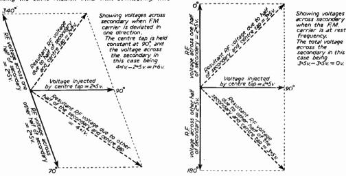
Fig. 2(c). How the detector works.
