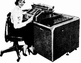
The "baby main"—the first desk-sized computer seen on this side of the Atlantic. It is designed to solve problems which are too complex for efficient solution on desk culculators, but too small for economical solution on "giant brains." This is a Burroughs machine,
