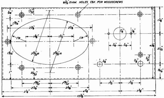
Fig. 7. - Details of the metal containing cabinet.
