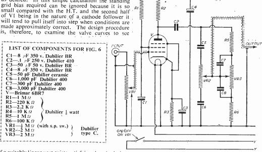
if a suitably linear part exists satisfying the stipulation that two-thirds of the H.T. should be dropped across the load and if this is so and there is some doubt about the conditions of working when the amplifier is built it is only necessary to insert a meter to check the current flowing through the second half to see if it conforms to the design figure decided upon, adjusting R3 if necessary to obtain correct conditions.
