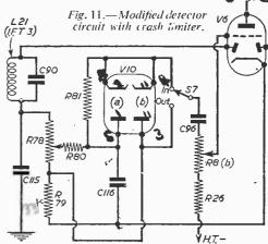
ADDITIONAL COMPONENTS (Fig. 11) R78-66 K Potentiometer Carbon. -R79—33 K 10% Erie Type 9. – R80 —680 K 20% Erie Type 9. R81—560 K 20% Erie Type 9. C115—100 pF Mica 20%. C116—0.1 #F 350 v. 20%. S6-S.P.D.T. Toggle Switch. V10-6H6. Note.—All other components included.
