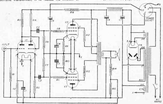
Fig. 5.—The amplifier described here. A list of parts appears on the page 565.
