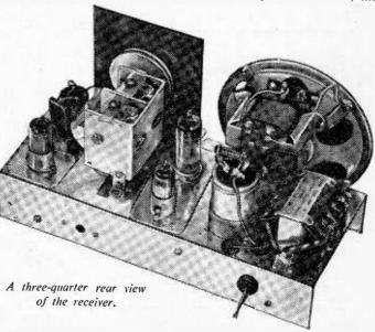
path along R12 provides bias for the triode section whilst the path R12+R13 provides bias for the pentode output section. The cathode by-pass condenser C12 (500 µF 12 v.w.), is unusually large, but is highly desirable from the point of view of stability. The anode of the triode section is fed from R10 (220 K) and the signal passed by C11 to the
