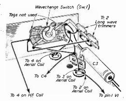
Fig. 4. — Further wiring details. See also Fig. 2.
