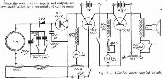
ted, but if desired, try one for the first transistor with high resistors by connecting a 1,000-ohm potentiometer between the OC70 emitter and battery positive.
