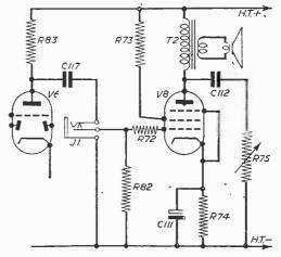
Fig. 13.—R.C. coupled output stage.
