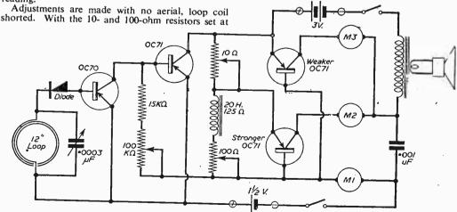
Fig. 6 (A). — An improved direct-coupled circuit.
