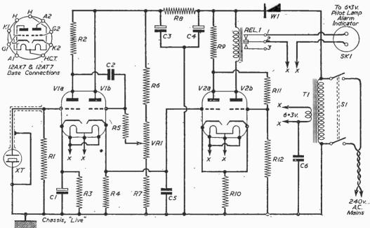
Fig. 1.—Theoretical circuit. A full list of parts appears on page 524.
