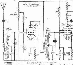
Fig. 1.—Theoretical circuit
