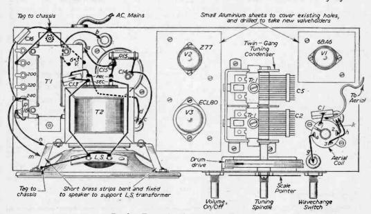
Fig. 2. -Top and underside wiring diagrams.
