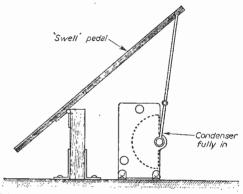
The Control "Off" or in the position of minimum volume.
