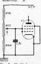
Fig. 9.—Modified screen circuit of R.F. amplifier.
