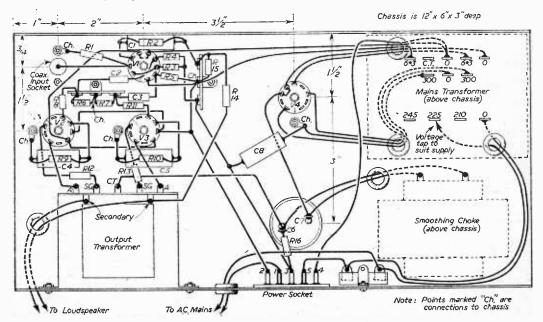
Fig. 7.—Layout and wiring of the amplifier.
