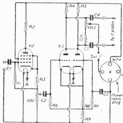
Fig. 4.—The "Y" Amplifier showing sync
