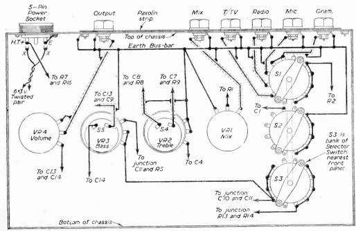
Figs. 10 and 11.—Top and below chassis wiring diagrams of the tone-control pre-amplifier.
