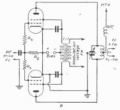
Fig. 1B.—Another circuit for balanced modulation.
