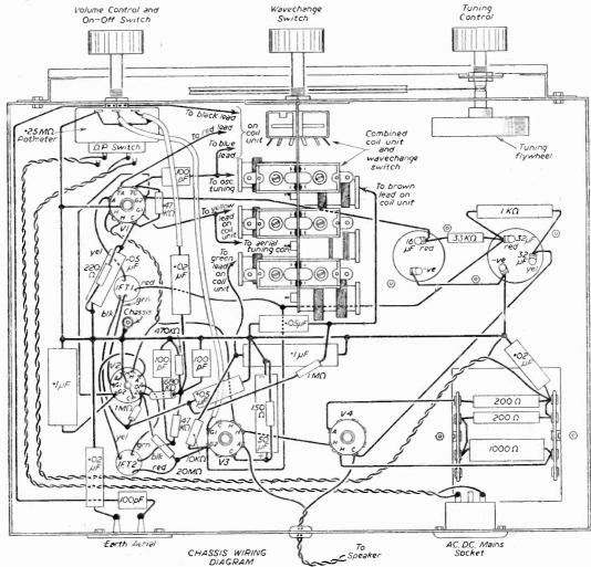
Wiring diagram of the A.C./D.C. Coronet Four.
