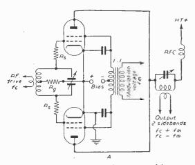
Fig. 1A.—One circuit for a balanced modulator.
