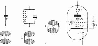
Figs. 1 and 2.— A diagrammatic explanation of inductance and capacity and "strays" in a valve.
