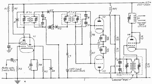
Fig. 7.—An experimental S.S.B. exciter unit. (A list of values will be found on p. 122)
