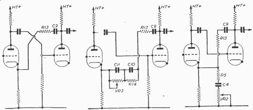
Fig. 4.—Circuit analysis at middle frequencies.
