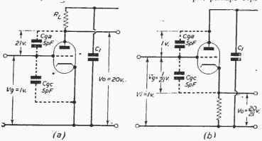
Fig. 9—A non-feed-back amplifier stage showing the stray capacities and their effect.
