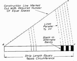
Fig. 2.—Diagram shows method of constructing a stroboscope for the rim of a turntable. The construction line AX is marked out with as many divisions as there will be bands (black plus white). X is the last point marked out. Join X to Y, and draw lines parallel to XY through each mark on AX.
