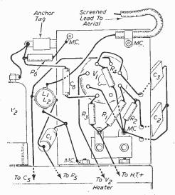
Fig. 10.—Wiring of underside of VI platform.
