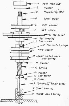
Fig. 7.—Full details of the take-up spindle.
