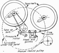
Fig. 5.—Layout of a tape recorder using a gramophone motor.
