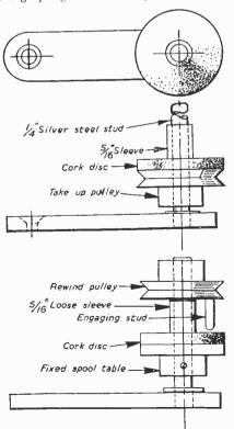
Fig. 3.—The feed-spindle with rewind pulley.
