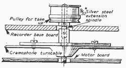
Fig. 1.—Method used to extend spindle of motor in the first recorder.
