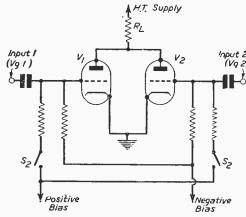
Fig. 1.—Basic Electronic Switch Circuit.
