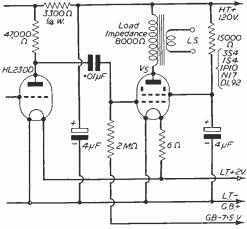
Fig. 3.—Recommended operating conditions for  $V_5$ , 3S4, 1P10, DL92, etc.
