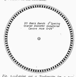
Fig. 1.—Laying out a Stroboscope for a turntable running at 33\frac{1}{33} r.p.m. under lighting from 50 cycles mains.
