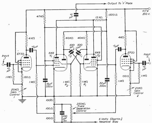
Fig. 4.—Complete circuit of the Electronic Double-beam Switch.
