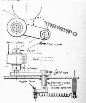
Fig. 2.—The pressure roller with toggle action.
