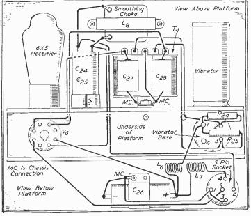
Fig. 9.—Wiring details of the power pack.
