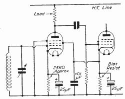
Fig. 3.—Circuit for anode-bend system of detection. Note that the screen voltage may be taken as shown.
