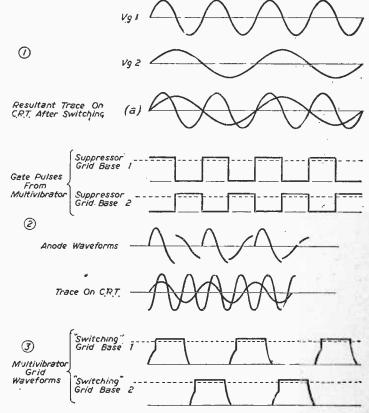
Fig. 2.—Waveforms associated with electronic switch circuits. (Not to scale.) (1) Simple circuit. (2) Gate circuit. (3) Triode-Hexode (anode wave-forms as in (2)).
