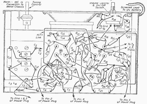
Fig. 8.—Wiring details of the main receiver portion.
