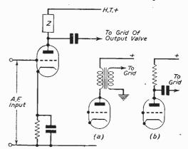
Fig. 1.—Basic circuit of triode amplifier, together with (a)—Transformer coupling, and (b)—Resistance-capacity coupling.
