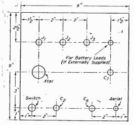
Fig. 4.—Details for panel drilling.
