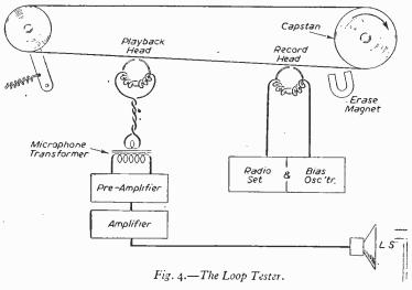
the other for playback, instantaneous checks can be made with different bias and recording current levels. It is most important to see that the heads are aligned correctly with one another, otherwise there will be a serious loss of top response.
