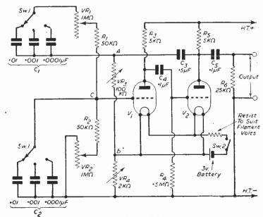
three-way Yaxley switch, while VR1 and VR2 are continuously variable resistors, ganged or geared together. (It so happens that at the time of writing a very suitable component, consisting of a pair of 1-megohm carbon potentionneters, mounted on a common spindle, is offered at 2s. 6d. by Radio Clearance, Ltd., of Tottenham Court Road, London, W.1.)
