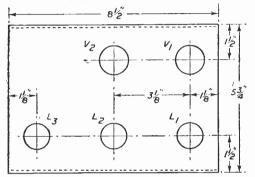
Fig. 2.—Chassis drilling data.
