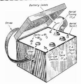
Fig. 3.—Appearance of finished unit.
