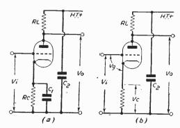
Fig. 2.—Simple amplifier and modification to introduce N.F.B.
