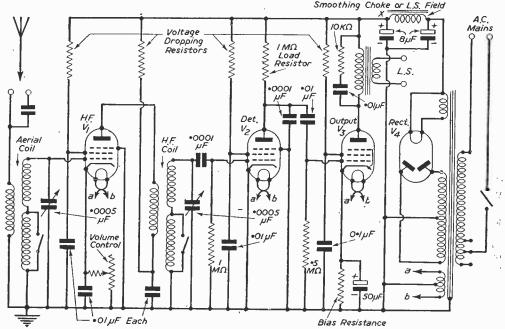
Fig. 1.—A suggested circuit for a simple 3-valve plus rectifier A.C. Mains Receiver. Details of design and the principles involved will be described in this series.
