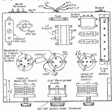
Fig. 2.—Chassis and Component layout.
