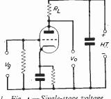
Fig. 4.—Single-stage voltage amplifier.
