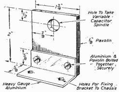
Fig. 5.—Bracket for condenser.
