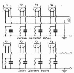
Figs. 1 and 2.—Note the possible difference of potential between heater and cathode of V4 in each
