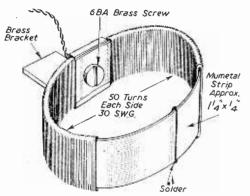
Fig. 1.—A simple record-playback head.
