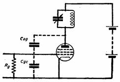
Fig. 3.—Method of varying the applied frequency.
