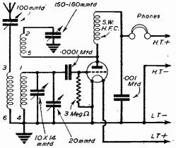
Fig. 3 .- Theoretical circuit of DX 1-valver.
