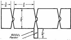
Fig. . . - The Sterba aerial. Its directivity can be increased by the use of additional half-wave sections. A reflector may be placed a quarter-wave behind the aerial to render, the system unidirectional.
