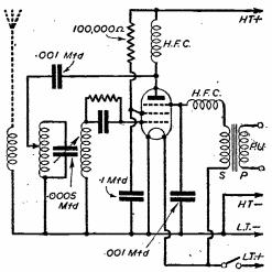
Fig. 4.-Suppressor grid modulation.
