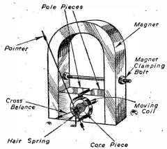
Fig. 1.-Diagrammatic view of a moving coil meter.
