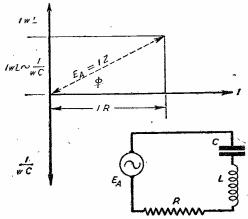
Fig. 2.—A simple A.C. circuit, and a vector diagram used to illustrate the meaning of power factor, which is dealt with in the reply to question two.
