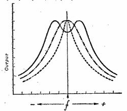
Fig. 1.—Different types of resonance curves for tuned circuits. That shown by a broken line is for a sharply tuned or loose-coupled circuit, that in a chain line is for a critically tuned circuit, while it double-humped curve shown as a full line is the ... Kilt of the coupling being too tight.
