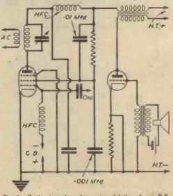
Fig. 6.—Combined anode and screen modulation of an R.F. pentode. The two condensers in the screen circuit form an A.F. potentiometer; values assigned are very approximate.
