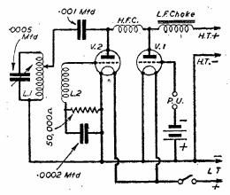
Fig. 6.—Circuit suitable for pick-ups with small output.
