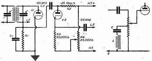
Fig. 3. (Left).—A noise-suppression circuit used between the second detector (V.I) and L.F. amplifier of a superhet receiver. Fig. 4 (Right).—A simple tune-connected audis volume centre consisting of a condenser C and choke L connected in series between a tapping on the volume control potentiometer and the earth line.
