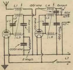
Fig. 1 .- Quench-operated circuit for U.H.F.
