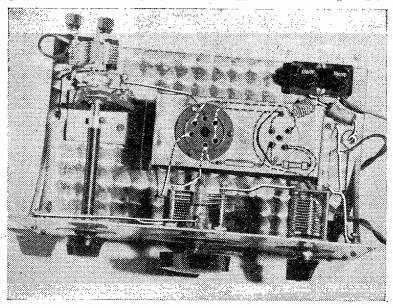
Fig. 4.—Top of chassis view of DX 1-valver.
