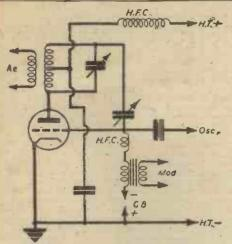
Fig. 3 .- A grid-bias-modulated R.F. amplifier.
