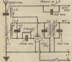
Fig. 3 .- Single valve quench-operated receiver:
