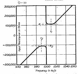
Fig. 5.—Input resistance variation as the input frequency is varied above and below resonance.
