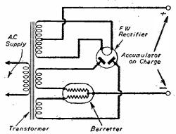
Fig. 2-Typical circuit for battery charging.
