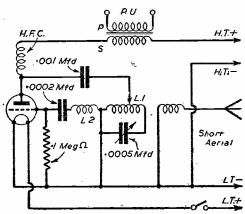
Fig. 3.—Simple tuned anode transmitter.
