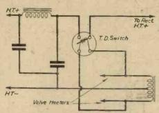
Fig. 1.—Connections for a thermal-delay H.T. The heating resistance may be fed from shown, or from the rectifier-heater winding, when this is provided.
