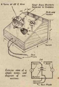
meter. To test the wiring of sets use the bulb by switching to the bulb on the panel. The battery is of the flat type 4.5 volts.—A. G. S. Cobb (Tamworth).
