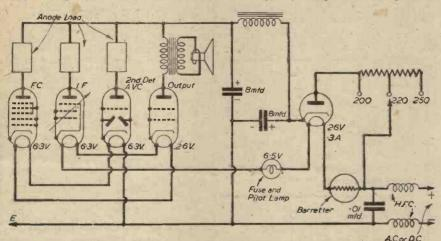
Fig. 4.—This skeleton circuit shows the arrangement of the heater wiring and rectifier connections in a typical superhet receiver of the AC/DC type. The tapped resistor in the anode creuit of the rectifier is not always necessary, and the combined break-circuit fuse and pilot lamp is an optional fitting.
