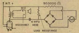
Westinghouse instrument-type rectifiers may be used up to frequencies of more than 100 kCs, and enable a simple and robust output meter to be constructed for such purposes as assisting trimming, measuring frequency response, etc. Full details for constructing such a meter are given in descriptive pamphlet No. 11b/1.
