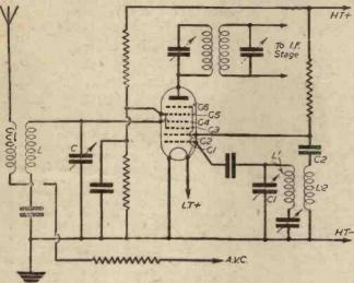
Fig. 1.—Circuit of octode frequency changer.
