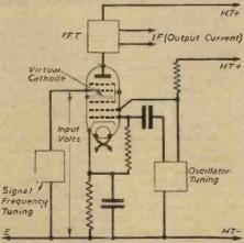
Fig. 1 .- An outline diagram of pentagrid frequency changer which helps to illustrate the meaning of conversion conductance—the ratio of I.F. current to signal or R.F. volts.
