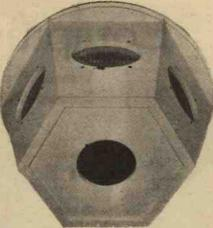
Fig. 4.—A multi-directional loudspeaker using several speaker units.
