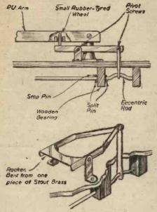
Details of an efficient pick-up lifting device.
