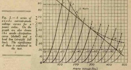
line we must avoid the curved portions of the  $I_a-V_g$  curves, where marked distortion would occur. It will be seen from Fig. 2 that point Z is nicely above the curve in the  $V_g=-40$  curve.
