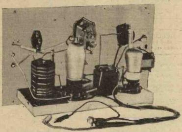
Rear view of the oscillator unit, showing the layout of components.
