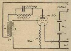
Fig. 1.—The oscillator circuit.
