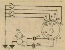
Fig. 2.—A selector system incorporating a reversible electric motor.
