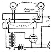
Circuit diagram for a novel house telephone system.
