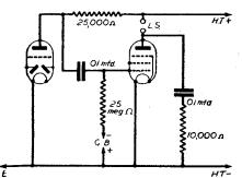
Fig. 3.—Skeleton circuit of an R.C.C. following a double-diode-triode. Fixed stage Fixed tone compensation is shown, and the connections given are for battery bias. Auto-bias may generally be used, as in Fig. 2.
