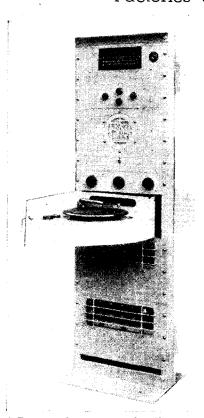
A Tannoy rack equipment with a 50-watt output stage and including provision for radio or record programmes.
