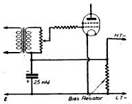
Fig. 2.—How automatic bias may be applied in the circuit shown in Fig. 1.
