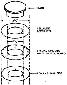
audio oscillator and a suitable null detector are connected to the meter, and the various frequencies, starting with 25 cycles, successively balanced out, a reference point and number being pencilled lightly on the dial at each null position. For reasons stated earlier, it is strongly recommended that the null detector used in this calibration be a valve voltmeter. The auxiliary resistor, R2, should be adjusted as needed to provide a more definite minimum indication.
