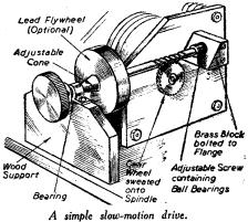
gearing mechanism can be used to give reduction ratios, the scheme I various have adopted being as shown in the sketch. The lead flywheel has been left on the shaft, as this appears to give additional control, and keeps the condenser stable at any given setting. The other end of the condenser shaft is carried through the panel to the tuning dial, the tuning knob being chassis.-L. A. JACKSON on side of (Narborough).
