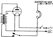
Fig. 2.—If preferred an audio-frequency oscillator, with the circuit shown here, may be used for practice purposes.
