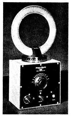
The radio compass unit made by Western Electric.
