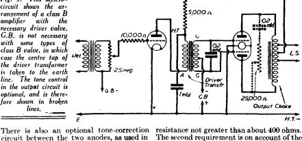
The second requirement is on account of the fluctuating grid current which it has to pass. In the case of both driver transformer and output choke (if used) it is of paramount importance that good-quality components, specially designed for Class B, be employed. Poor transformers have a more profound effect on the output from Class B than they have on that from a single-valve or even a Class A push-pull output stage.
