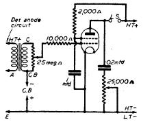
Fig. 1.—The circuit arrangement for an efficient transformer-fed tetrode output circuit suitable for about 500 mW. output.
