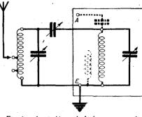
Fig. 4.—A suitable method of connecting the unit to a single tuned aerial circuit to provide band-pass tuning.
