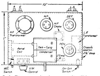
Fig. 3.—The more compact form of construction made possible by using a metal or metallised chassis. As in Fig. 2, dimensions are approximate only and components are not of any particular make or type.
