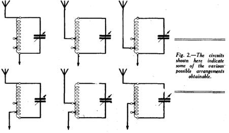
provide a fair number of alternative effects, the coil be tapped at one-fifth and twofifths of the distance from one end. This will then provide a number of alternatives as indicated in the diagrams. An alternative method of connection is to add the unit in parallel with the receiver, that is, with the aerial and earth leads connected to the receiver in the usual way, but with duplicate
