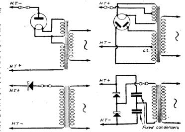
Fig. 2.—Diagrammatic circuits for four different types of widely-used rectifier arrangements.
