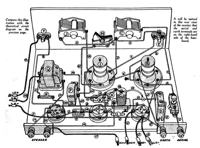
Fig. 2.-Perspective lay-out of the circuit given in Fig. 1.
