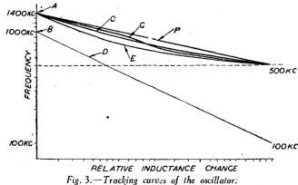
oscillator is approximated in the response curve E, which indicates the result obtained when a shunt trimmer inductance 9 is employed in conjunction with the main oscillator winding 4 in the arrangement shown in Fig. 2.
