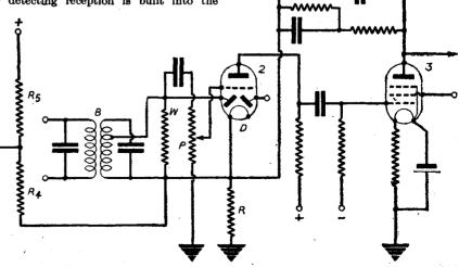
Fig. 2.—The circuit arrangement where a diode is used for detection.
