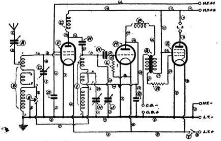
Fig. 1.—Theoretical circuit diagram of a three-value receiver.
