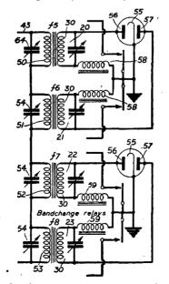
Fig. 3.—A more sensitive arrangement for the receiver.
