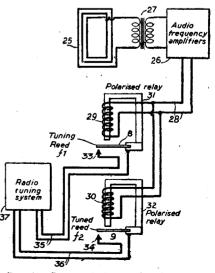
Fig. 6.-Circuit of the tuned-reed receiver.
