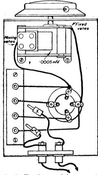
Fig. 5.—This plan view of the unit reveals the simplicity of construction and wiring.
