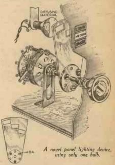
aluminium mask inserted in between (see diagram). All that remains to be done is the final adjustment of the mask to illuminate the correct apertures at the appropriate band.—D. Guerin (Lambeth).
