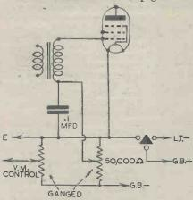
Fig. 1.—An experimental method of combining variable-mu volume control and grid bias control.
