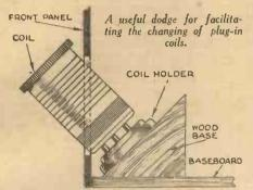
in the front or side of the set and to screw the coil holder on to a wooden mount in the position shown. The top of the coil then protrudes at the front or side of the receiver, whichever arrangement suits best. This allows the coil to be changed without difficulty, but needless to say it applies only to plug-in coils.—A. Cook
