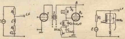
Fig. 6.—Illustrating the resonance short-circuit feature.
