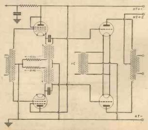
Fig. 8.—Typical example of cathode coupling to positive grid drive "Class B" push-pull stage.
