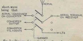
Fig. 2.—Diagram of connections for a three-pole anti-capacity switch.
