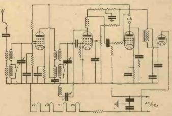
A three-valve circuit of the H.F., Det. and Pentode output class for universal mains operation. A throw-out aerial is used.
