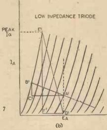
Power output proportional to areas of triangles:  $A^1B^1C^1$  ... Class A (bias at  $A^1$ ) ... Class A (bias at A<sup>1</sup>)
