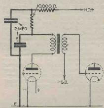
Fig. 1.—(Left) The most simple form of anode de-coupling. If this does n result then the method on the right should be used. If this does not produce the required
