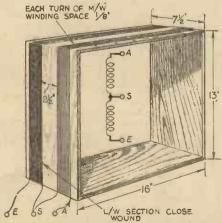
Fig. 3.—Shows the winding data and theoretical circuit for the frame aerial. A to S, med. waves, 14 turns 26 s.w.g.; S to E, long waves, 40 turns 32 s.w.g.
