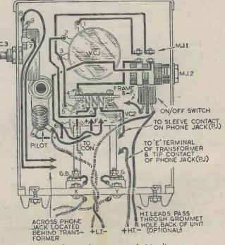
Fig. 4.—Layout of components and wiring diagram.
