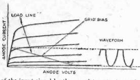
Fig. 12. (Left)—Form of distortion with pentode, resembling current distortion.
