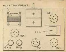
Fig. 2. - A suggested layout, showing how the mains equipment is located to one side of the chassis away from the coil.
