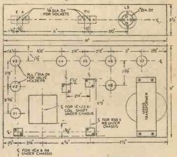
Fig. 4.—Chassis construction and drilling details.
