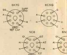
Fig. 2.-Pin connections for the valves. Note
