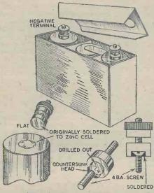
A method of utilising old battery terminals.
