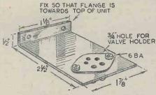
Fig. 3.—Details of valveholder bracket.
