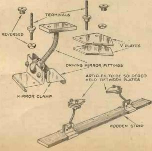
A novel clamping device for holding work while soldering.
