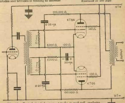
Fig. 11.—Typical circuit for power tetrodes in push-pull, employing negative feedback.
