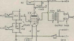
Fig. 1.—Theoretical circuit diagram of the combined pre-amplifier and mixer unit.
