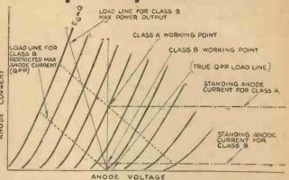
Fig. 5.—Comparison between Class A and two alternative applications of Class B, the one alternative for maximum economy in average anode current ("Q.P.P."), and the other alternative for maximum power output (low impedance loading "Class AB1")
