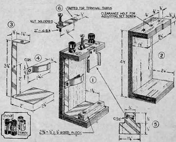
An adapter for charging dry accumulators and torch cells.
