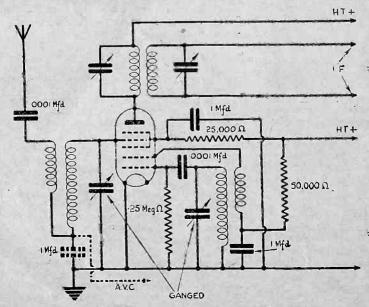
Fig. 2.—The pentagrid or heptode frequency-changer is probably used most extensively at the present time. It is efficient on all wavebands down to about 20 metres, but in some cases an additional triode should be used as sepa-rate oscillator.
