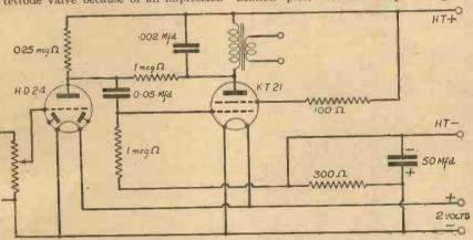
Fig. 10.—Typical circuit for a 2-volt battery power tetrode employing negative feedback.
