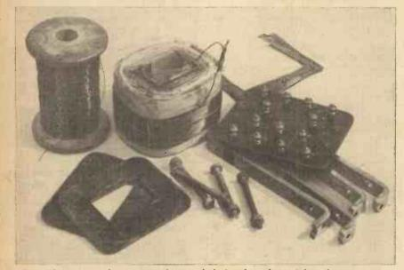
Parts of a commercial mains transformer which has been dismantled to show construction. Note insulation between layers of windings.
