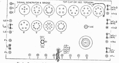
Fig. 1. Front view of the tester, showing layout of valveholders and sockets.
