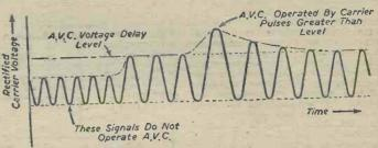
Fig. 4.—Delayed-automatic volume control, as shown here, is a well-known application of amplitude difference acting as a discriminator.
