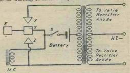
Fig. 2.—Basic non-synchronous vibrator circuit.
