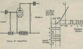
Fig. 8.—If this type of circuit is employed, then only pulses exceeding a certain amplitude will be passed.
