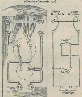
Fig. 4.—Details of wiring, and theoretical circuit.
