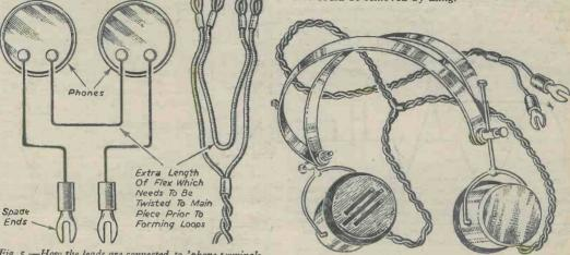
Fig. 5 .- How the leads are connected to 'phone terminals, with view showing methods of twisting the leads together.
