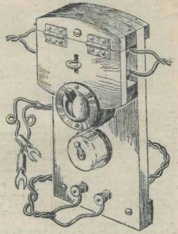
Fig. 6.—The completed charging board.
