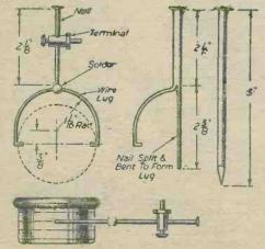
Fig. 3.—How the 'phone lugs are made up from wire or a nail, with side elevation.
