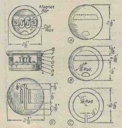
Fig. 1.—Top view, sectional side view, with details of cover piece and case parts.
