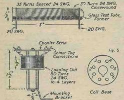
Fig. 4 (above) and Fig. 5 (right).—Constructional details of the chokes and coil base connections.
