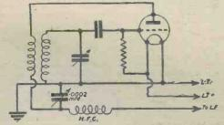
Fig. 4.—This arrangement is known as "throttlecontrolled reaction."
