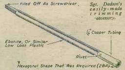
tubing around the nut's sides, withdrawing it when finished with by screwing in the appropriate bolt and fastening it in a vice.
