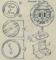
Fig. 2.—Case ring, diaphragm and cover flange sizes, with top plan showing wire connections, plus detail of coil top and bracket.
