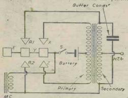
Fig. 3.—Basic synchronous vibrator circuit.
