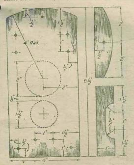
Fig. 1.—Details of mounting board, with back end pieces.
