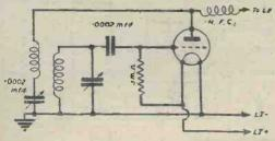
Fig. 1.—The simplest reaction arrangement.
