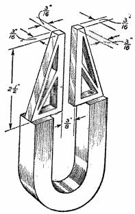
Fig. 4.—Suggested construction of microphone. Essential dimensions are given.
