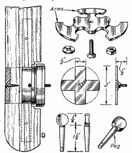
Fig. 3.—Enlarged detail of body, showing how earphone fits in its recess, with details of diaphragm and wooden
