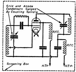
Fig. 4.—Heterodyne frequency meter.
