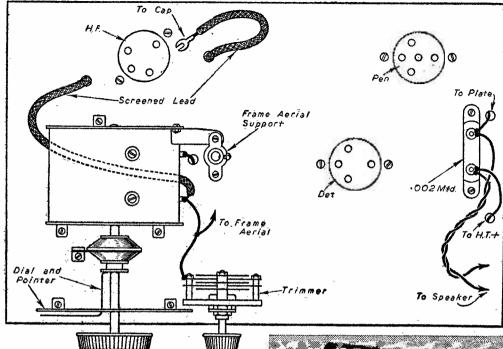
Fig. 2.—Top of chassis layout.
