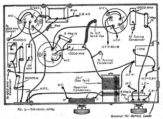
get the circuits in tune. The trimmer connected to the frame is of rather large capacity, and should not need much adjustment throughout the tuning range. Two separate tuning condensers were employed in place of the gang condenser and trimmer originally. This removed any ganging difficulties, but it was found later possible to use a twin condenser instead.
