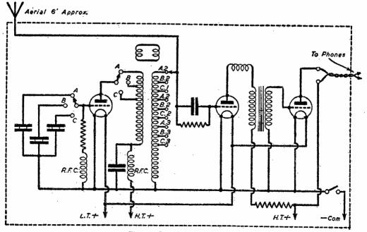
Fig. 5.—Crystal frequency monitor.
