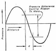
Fig. 3.—Illustrating principle of "Velocity" operation.
