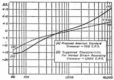
Fig. 1.—Characteristic curves for recording crossovers.
