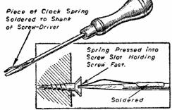
Adapting a screwdriver for holding screws in awkward places.
