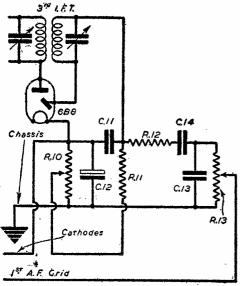
Fig. 1.—Modified circuit for the noise limiter.
