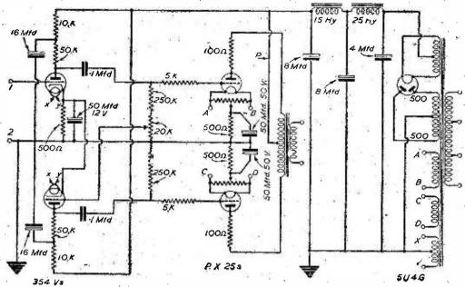
Fig. 3.—Circuit of well-known conventional type amplifier.
