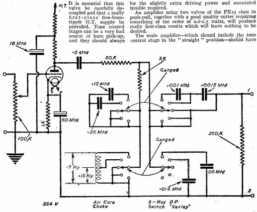
Fig. 2.-Tone control circuit.
