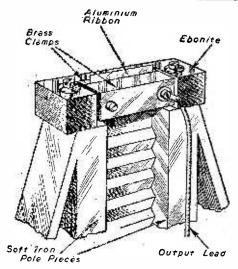
Fig. 5.—Suggested construction of end clamps.
