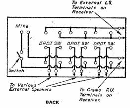
The board is shown wired for three external speakers, but any number can be fitted, an extra D.P.D.T. switch, in parallel with the rest, having to be added for each L.S. A sensitive headphone may be used in place of the microphone, if desired.
