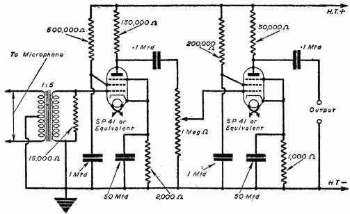
Fig. 7.—Suggested circuit diagram for microphone amplifier.
