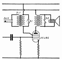
Fig. 7.—Diagram of intervalve transformer and switching arrangements and diagram of base connections.
