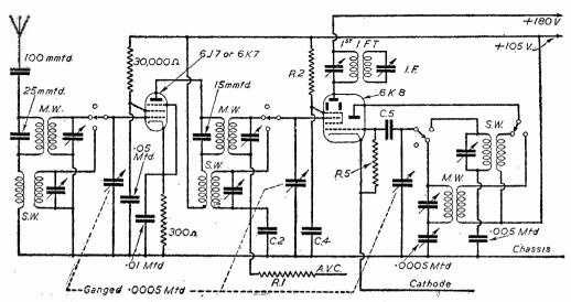
Fig. 3.—Circuit diagram, showing H.F. stage with suitable switching for medium wavelength,
