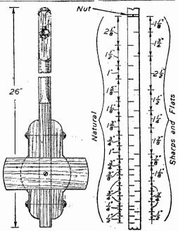
Fig. 4.—A back view and diagram showing how finger-board is marked to give the usual "fret" positions.
