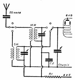
Fig. 4.-Modified R.F. circuit.
