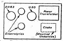
Fig. 3.—Chassis, showing position of main components.
