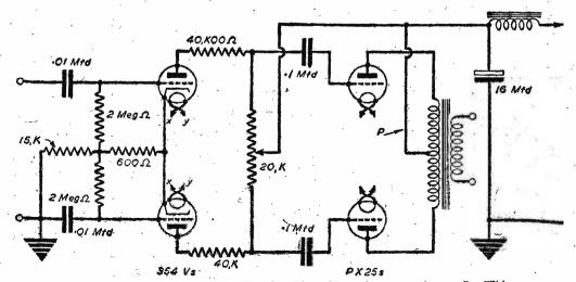
Fig. 4.—Alternative input (Schmitt circuit). To balance, in each case, insert 50 resistor at P. input balance 20 k. potentiometer to minimum signal—with 'phones across P. With 1,000 c.p.s.
