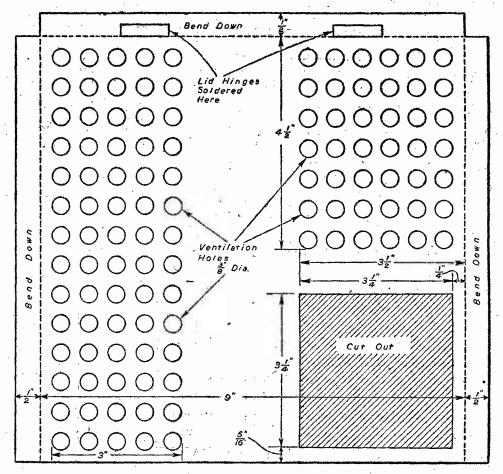
Fig. 4.—Rear view of chassis, showing ventilation holes.
