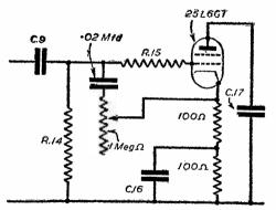
Fig. 2b.—Circuit diagram for "bass boost."
