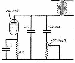
Fig. 2a.-Circuit for "top cut."
