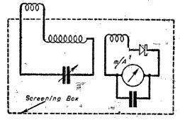
Fig. 2.-Modern absorption wavemeter.
