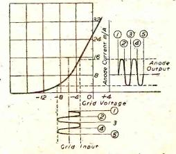
Fig. 2.—This diagram shows how the anode waveform can be projected geometrically from the grid input waveform on an anode current-grid voltage curve.
