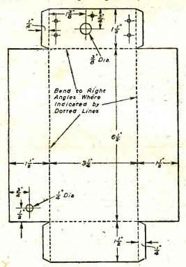
Fig. 3.—Plan and dimensions of case. Fold on dotted lines.
