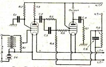
Fig. 1.- Theoretical circuit showing high- and low-note boosters.
