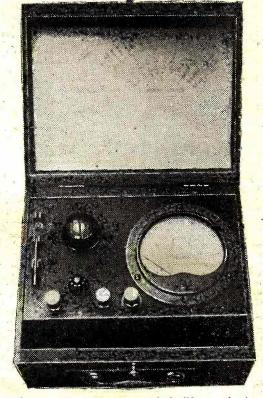
Front view of the multimeter, with the lid open, showing the panel and control knobs.
