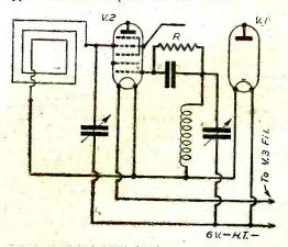
Fig. 3.-Circuit diagram of frequency-changer connections.
