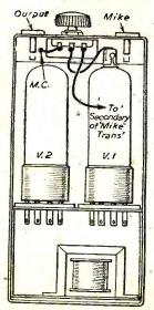
Fig. 2.-General assembly of the amplifier in case.
