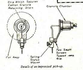
fixed the stylus to the piston, in the granule chamber. This head was used on an aluminium arm, the complete assembly being very light. A transformer (to be found in the base of these microphones which are sold, at about 6s. 6d. each) and battery are, of course, necessary. Background hiss was very slight indeed, and quite unnoticeable while playing .- D. C. SWAINE (Tengerden).
