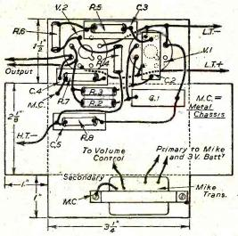
Rig. 4.-Wiring plan and flat shape of valveholder platform.
