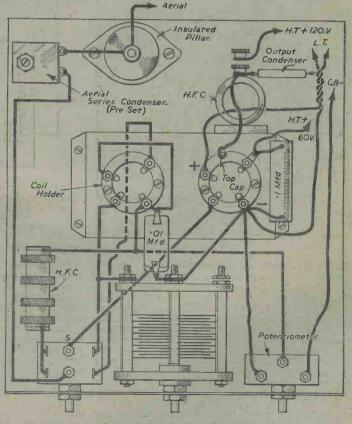
Fig. 2.—Wiring diagram and component layout of the S.W. H.F. unit. The coil and valve-holder platform allows the critical wiring to be kept short.
