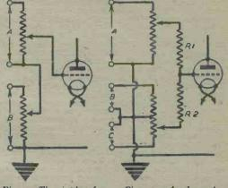
Fig. 3 .- The simplest form of mixer circuit, suitable for two inputs. Provides volume control, fading and mixing.
