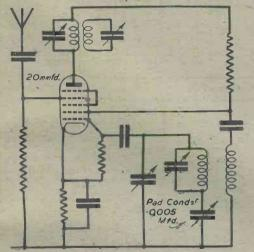
Fig. 4.—Circuit used for testing oscillator coils. A triode hexode can be used.
