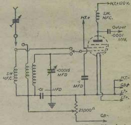
The circuit of the variable Mu H.F. amplifier, showing how a tuned or untuned aerial circuit is obtained by switching.
