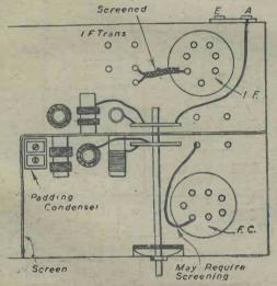
Fig. 1.-Lay-out of frequency changer stage, with small sub-chassis coils.
