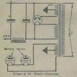
connected them to the heater winding of the transformer as the winding was 4 volts and the valves were 2 volts each, and in series, the voltage was perfect. You will see what I mean by my circuit above. The set works quite well.—J. M. T. WOOD (Enfield).
