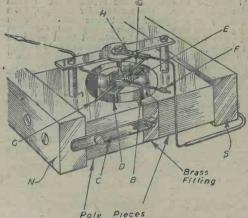
Fig. 1.-Moving coil meter movement.
