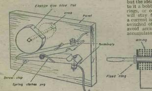
A simple L.T. switch made from odds and ends.
