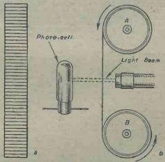
Fig. 3.—How a narrow strip of paper marked by horizontal lines may be electrically transmitted to a distance receiver.
