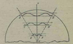
Fig. 4.—Showing how the waveform is compressed as the recording approaches the centre.
