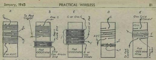
Fig. 7.—Coil details (see table). A, medium-wave aerial coil; B, medium-wave oscillator coil; C, long-wave aerial and oscillator coil; D, s.w. aerial coil; E, oscillator as aerial coil.
