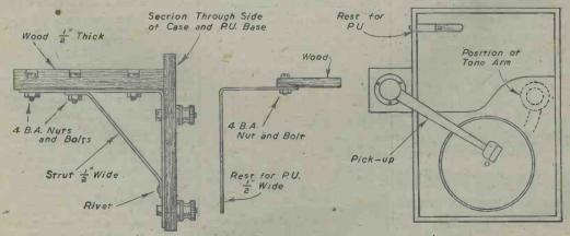
Method of fitting pick-up to portable gramophone. E. W. Bull (Southsea).
