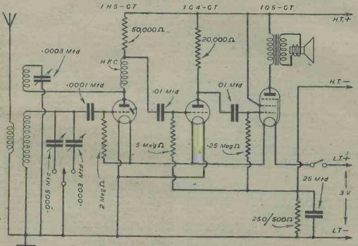
Fig. 1.-Circuit for a simple and very compact three-value all-dry receiver.
