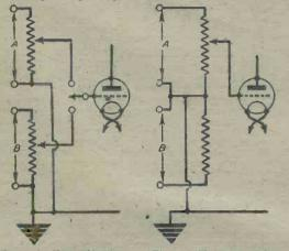
Fig. 1. - Two distinct input circuits, each having their own volume controls. Only suitable for switching from one circuit to another. No mixing. Fig. 2.—No switching required as use is made of a "fader" type volume control. This allows fading from one input to another but not mixing.
