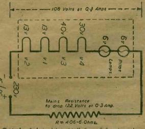
Showing how the heater chain is virtually " across" the mains supply.
