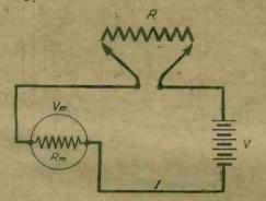
Fig. 1.—The basic circuit illustrating the principle of the ohm/volt meter.
