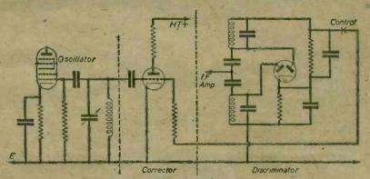
Fig. 4.—Skeleton diagram showing the general arrangement of a simple system af automatic frequency correction.
