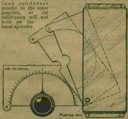
Fig. 2.-The 49 m. card in position ready for calibrating. Remaining card s swing back into pocket as shown .
