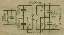
Fig. 5.—Circuit of amplitude discriminator.
