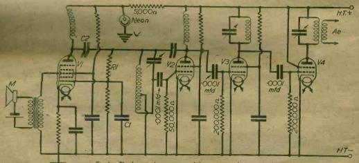
Fig. 1.—The theoretical arrangement of the transmitter showing the voltage stabiliser across the oscillator's H.T. lead.
