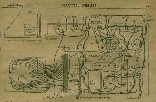
Fig. 4.-Layout and wiring of power unit. The L.T. voltage adjustment panel is accessible from side of panel as shown by the inset.
