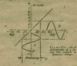
A carrier-wave whose frequency varied as shown at A would produce an AF output as shown at B, which, in this case, is a perfect reproduction. We now have to find a device that has a characteristic
