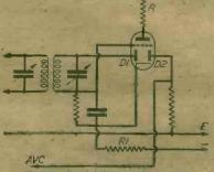
Fig. 3.—Simplified circuit of a second detector providing delayed and ampli-fied A.V.C.
