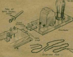
A simple arrangement for a detachable morse key and oscillator.
