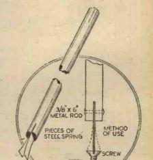
A useful tool for holding and driving screws in awkward corners.
