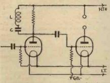
Fig. 9.-L.C. is an acceptor luned to 5000/6000 cycles for use as a heterodyne whistle filter.
