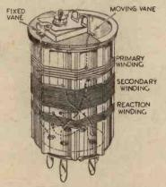
method of incorporating an aerial condenser with a plug-in coil.
