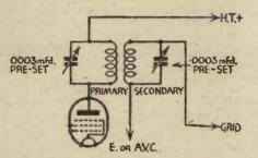
Fig. 2.—Connections for the transformer shown in Fig. 1.
