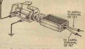
General view of a simple electro-magnetic switch.
