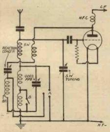
Fig. 3.—A variation of the circuit shown in Fig. 1, where reaction is used on all wavebands.
