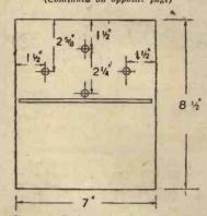
Showing all dimensions for drilling and location of panel components.
