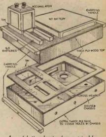
A novel battery-housing box contrived from an old wooden chassis.
