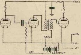
Fig. 1.—A normal L.F. circuit showing how the bias is applied to the grids of battery-operated values.
