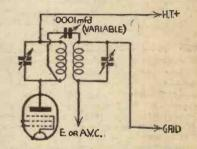
Fig. 3.—How to obtain variable selectivity, by means of a small variable condenser.
