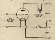
Fig. 3.—Circuit diagram of the one-valve amplifier, which should be constructed to match the B.F.O. unit. In operation four 9v. grid-bias batteries form the H.T. supply.
