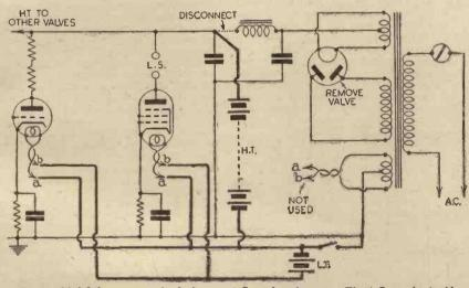
Fig. 1.-Modified connections for feeding an A.C. set from batteries. The A.C. supply should. of course, be disconnected, in which case it is not essential to remove the rectifying valve.
