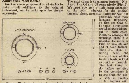
Fig. 1.-The front of panel, showing the three additional sockets.
