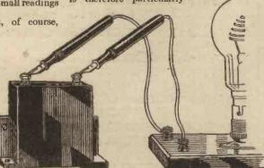
Fig. 4.-Testing the insulation of a fixed condenser by means of the neon lamp.
