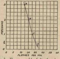
Fig. 7.—The curve used for finding the values of resistances.
