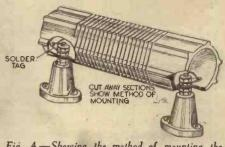
Fig. 4 .- Showing the method of mounting the tuning coil.
