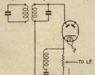
Fig. 8.-An I.F. by-pass to diode load in the second detector circuit of a superhet.
