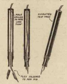
Fig. 3.—A method of making a test prod from an old fountain pen.
