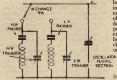
Fig. 1.—A normal arrangement of padders and trimmers in a superhet for medium and long-wave reception.
