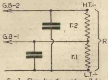
Fig. 3.—Shows how the resistance R has to be tapped to allow more than, one G.B. supply to be obtained.
