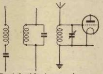
Figs. 1, 2 and 3.-A series tuned, or acceptor, circuit; a parallel tuned, or rejector, circuit; and an ordinary tuning circuit respectively.
