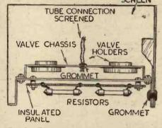
Fig. 5.—Further details of the metal chassis and assembly of parts.
