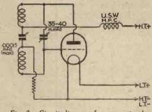
Fig: 2.—Circuit diagram of a conventional ultra-short-wave oscillator.
