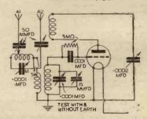
Fig. 2.-Circuit diagram showing an alternative method of aerial resonance tuning.
