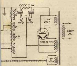
al scircuit of the monitor tube and power-pack unit.
