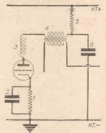
Fig. 1.—A meter included at the point marked will generally indicate the presence of a faulty component giving rise to crackles.
