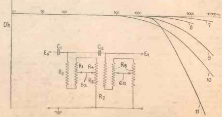
Fig. 3.-A bass cut fitter made up on the same lines, and Fig. 4.-Curves, showing the effect of the tone-control circuit referred to.
