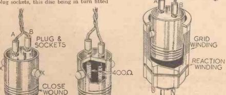
Figs. 3, 4 and 5.—Suggestions for coupling various aerials to standard short-wave coils.
