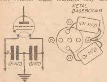
Fig. 1.—Condensers across the heater circuit as shown here should be used. The detector stage is usually best for this scheme.
