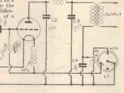
Fig. 1. — Theoretical circuit of the adapter as described on this page.
