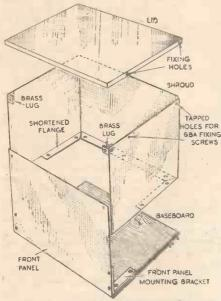
Fig. 4.—Details of the baseboard, panel, and screen-casing assembly.
