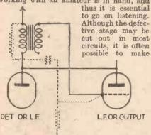
A. makeshift repair for a broken-down transformer.
