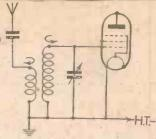
Fig. 2.—Here a separate aerial winding is used, this being in-ductively coupled to the grid winding.
