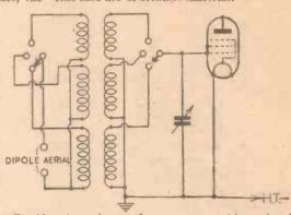
Fig. 10.-A satisfactory three-range tuner with aerial and grid windings.
