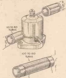
Fig. 5.—A simple but efficient home-made S.W. choke and a suggestion for improving an old choke
