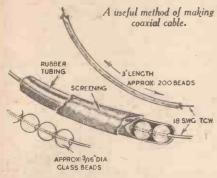
rubber tubing, as shown in the accompanying sketch, finally screening with some very wide (screened aerial lead) braiding.
