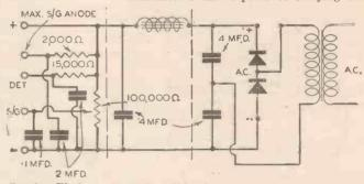
Fig. 2.—The basic circuit of an H.T. eliminator. The three sections are described in the text.
