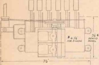
Fig. 3.—Over-all Clearance Dimensions.
