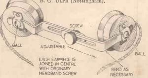
A simple method of converting headphones for use as a house telephone.
