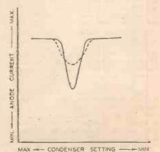
Fig. 3.—The curve is made symmetrical in the case of " doubler" and P.A. stages.
