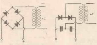
Fig. 1.—The Bridge circuit on the left and the Voltage-doubler on the right. Both give full-wave rectification.
