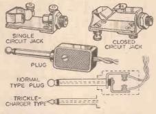
Fig. 1.—Two types of simple jack and also a complete jack plug. Below are shown the construction of the usual type of jack plug and of the special kind used for trickle-charger connection.
