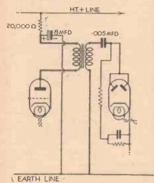
Fig. 3-Modifications necessary when using an insensitive pick-up.
