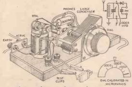
Pictorial view and circuit diagram of a condenser testing unit.
