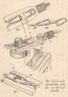
ends and bending to the clip shape being done finally. The inset (c) shows the spring fitment, also the filed "U" base in the cut-out portion of the brass mount, depicted by "F."
