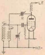
Fig. 6. (Left)-This reactioncircuit is identical in principle with the aerial-grid circuit shown in Fig. 2,
