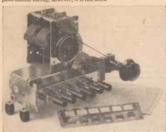
Fig. 1 .- The Complete Push-button Tuning Unit.
