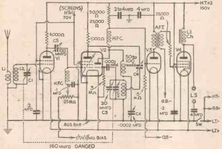
Fig. 1.—A suggested 4-valver built round the triode-pentode as H.F. and detector stage.
