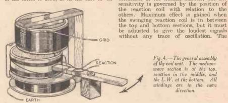
Fig. 4.—The general assembly of the coil unit. The medium-wave section is at the top. reaction in the middle, and the L. W. at the bottom. All windings are in the same direction.
