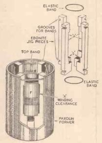
A method of centralising aperiodic coils.
