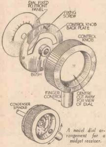
A knob of approximately 2in. diameter was taken, and the centre cut out, as shown. A semi-circular slot was cut from a disc of polished aluminium, and after fixing a bush to the centre the whole disc was screwed to the back of the control knob. A dial was made and stuck to the panel of the receiver in such a way as to show through the slot in the aluminium disc, with the addition of a small plug as a finger control easy reading of the dial was obtained.—
