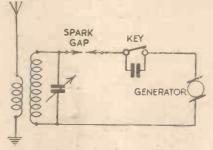
Fig. 1,-Representative diagram of a spark transmitter.
