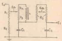
Fig. 2.—The theoretical circuit of the tone control arrangement. Values are given on facing page.
