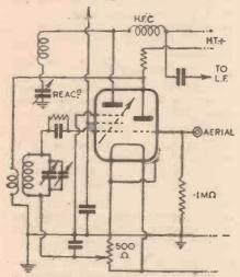
Fig. 3.—An H.F. and detector stage using a triode-pentode. The H.F. stage is untuned.
