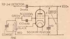
A B.F.O. stage built around the new Varley coil unit and the method of adjustment for panel control.
