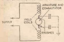
Fig. 2.—Typical diagram of a small electric motor-Suppressor condensers are shown by broken lines.
