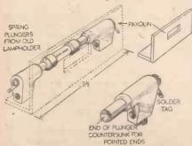
Spring plungers from disused lamp sockets were used for making these adjustable mounts for small components.
