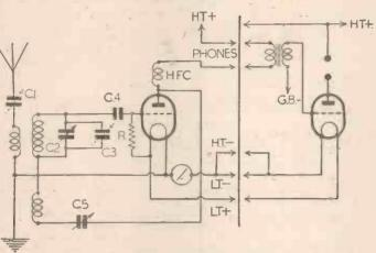
Fig. 1.—A standard short-wave circuit, showing how an L.F. stage may be added.
