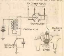
Fig. 3.—Simplified circuit of a car ignition sustem.
