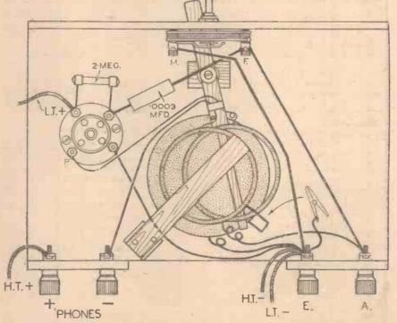
Fig. 2.—All wiring can be followed from this plan view. Keep components in the positions shown, as additions will be made next week.
