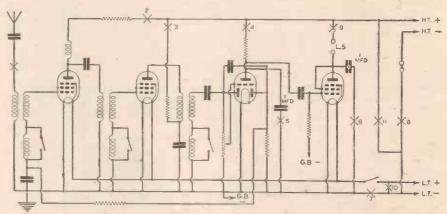
Fig. 4.—A simplified diagrammatic skeleton circuit used to show some of the points at which jacks can conveniently be included.
