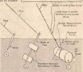
How to ensure firm anchorage for a wireless mast.
