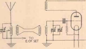
Fig. 2.—A link-coupled aerial tuning arrangement.
