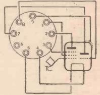
Fig. 4. - Pin connection data for the triodepentode.
