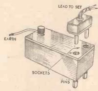
Fig. 5.—A convenient type of twin-condenser suppressor for connection in the mains supply to the set.
