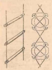
Fig. 1 Aerial feeders, or connecting links, as used for short-wave reception.
