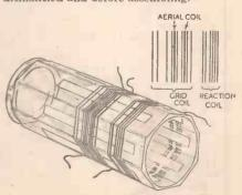
Fig. 4.—A novel method of making a low-loss self-supporting coil with 3 windings.
