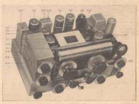
An inside view of the claborate Eddystone Model E.C.R. This is a 10-valve receiver which costs \$45 complete. The cabinet and controls may be seen at the top of the facing page.
