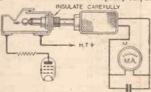
Fig. 3.—The method of connecting a closed circuit jack in a circuit where current measurements are to be taken. Since the jack is in the H.T. circuit care should be taken to insulate it from a metal panel or other earthed part.
