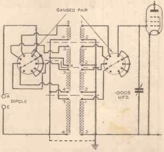
Fig. 2.—This circuit shows how a four-range tuner can be used with a double-pole five-way rotary switch. Connections are shown for a dipole aerial, but an ordinary aerial earth system can be used by making the connection shown by the broken line.
