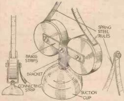
Flexible steel rules are used for this collapsible aerial
