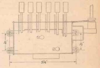
Fig. 2.—Dimensions for Mounting the Unit.
