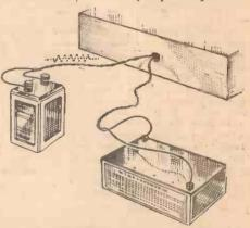
Fig. 2. Battery connections. Resistance in the L.T. leads can reduce efficiency.
