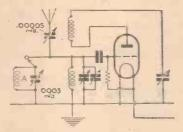
Fig. 1.—A simple method of aerial tuning.
