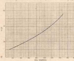
The curve of the "yellow" spot coil covers a waverange of 40 metres to 15.5 metres.
