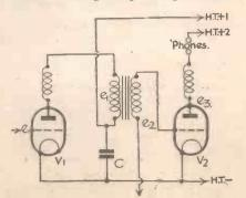
Fig. 2.-Circuit diagram incorporating a directly coupled transformer.
