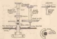
Operating band-spread and band-set condensers from a single control knob.
