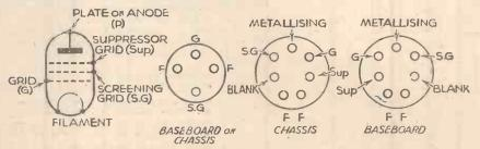
Fig. 5.—Details of the connecting points of H.F. valveholders and the electrodes of an H.F. valve.
