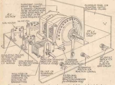
Fig. 1.-The suggested component layout for a combined R.F. and first L.F. chassis.
