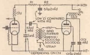
Fig. 5.—Suitable values for the various components are given in this illustration.
