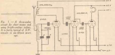
the vernier as a bandspread condenser. Whereas nowadays hand-capacity troubles would be largely overcome by suitable screening and the use of better tuning condensers, the desired result was (some-times) obtained then by attaching a very break beloits extension animals to the long bakelite extension spindle to the vernier condenser knob. Similarly, the control knob of the swinging-coil holder was provided with a long ebonite rod extending a foot or more from the knob.
