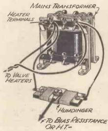
To remove hum a separate artificial centre tap may be provided in A.C. receivers as shown here.
