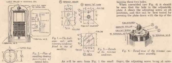
densers, results on the medium waveband were quite satisfactory. On changing over to the long-wave, however, I found that it was necessary to readjust the trimmers As will be seen from Fig. 1 the small trimmer is fitted to the top of the coil, and two leads taken (one from the adjustable plate, and one from the fixed plate) to terminals 3 and 6 respectively.
