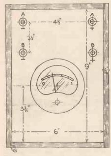
Fig. 2.—Panel layout and drilling dimensions.
