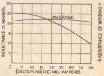
Fig. 4.—Illustrating the drop in inductance resulting in a badly designed choke using thin high-resistance windings.
