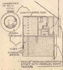
Fig. 4.—Diagram illustrating the pick up of interference and its effects.
