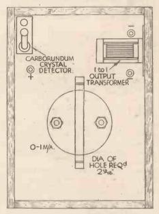
Fig. 3.-Component layout of the Output Meter.
