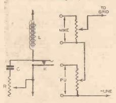
"click" fi Fig. Fig. 2.- A simple mental filter mixer input circuit. circuit.
