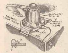
Method of fitting a removable pick-up to a portable gramophone.
