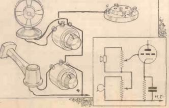
Fig. 2.—How to connect a "mixer" circuit made up with two separate volume controls.
