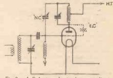
Fig. 2.—A P.A. stage showing how neutralisation is applied. Note the centre-tapped anode coil.
