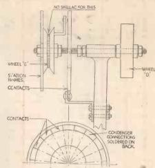
Fig. 5.-Illustrating a method of using the switch for push-button tuning.
