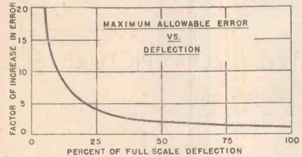
Fig. 2.—The maximum allowable meter error increases very rapidly for deflections less than one-third of full scale. To find the per cent. error, multiply the factor of increase in error by the per cent. rating of the meter.
