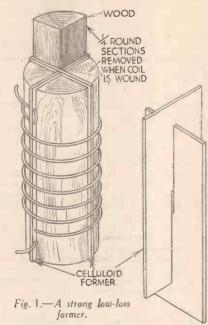
is advisable to carry out the winding of the coil while the tube is still in position as this allows easier handling of the celluloid
