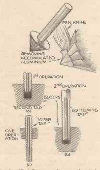
Fig. 5.—(Top) Removing aluminium deposit from a clogged countersink bit. Fig. 6.—Details of lapping.
