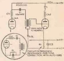
Fig. 3 .- Circuit diagram of a filter-fed transformer sustem.
