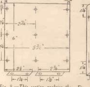
Fig. 8.—This section encloses the rear of the I.F. screens (Fig. 4) and is also attached to Fig. 7.
