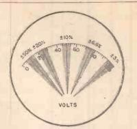
Fig. 1.—The shadow of doubt in a meter reading remains constant in width, but increases in percentage for decreasing needle deflections.
