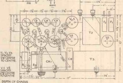
200-ohm, and 4.9 volts with a 500-ohm microphone. If the amplifier is to be used with a microphone not needing the polarising supply, R5 and condenser C3 may be dispensed with and resistance R1 then earthed direct.
