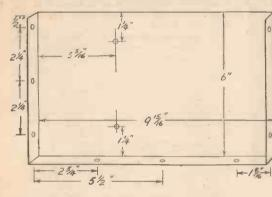
chassis and holder should suffice. Now comes the difficult part. On each of the comes the dimensi part. On each of the top condenser partitions mount one of the band-spread condensers, making quite certain that the lock-nut is tight and that all condensers are exactly in the same position; that is, with the fixed plates towards the bottom. Do the same with the hand extern retire the band-setters, noting their position from the illustrations given last week, and then
