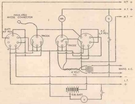
Fig. 2.-Details of a comprehensive tester for 7- and 4-pin valves-battery and mains.
