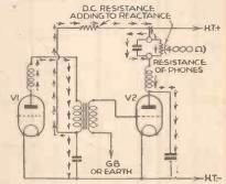
Fig. 6.—This diagram shows the main direction of current flow as explained in the text.
