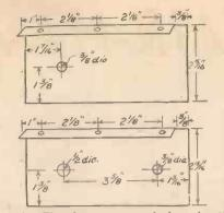
Fig. 3.—The above are two of the under-side partitions separating the band-setters. The third partition is shown in Fig. 10. The upper unit is placed nearest the rear of chassis, and the lower is mounted next to it.
