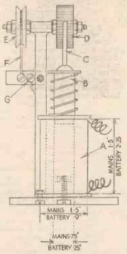
Fig. 1.—Side view of the completed electrically operated push-button switch.
