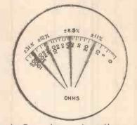
Fig. 4.—For an ohmmeter the possible errors are greater than those of the meter movement itself because of the non-linear scale.
