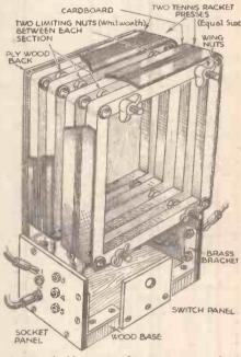
A pair of old tennis racket presses are used for this experimental frame aerial
