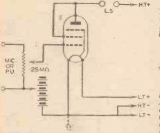
of unit that could be made is one with a single battery-operated valve. It can be built on a very small baseboard or in a compact wooden box, and can be carried about very easily. Small batteries can be housed within the container, so that the only external connections required are those to the microphone or pick-up and those to the loudspeaker.
