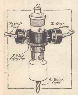
Multiple mains connections may be arranged in the workshop as shown here, but care must be taken not to overload the pendant flex.
