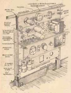
Fig. 1.—General idea of the method of mounting test components on a rack.
