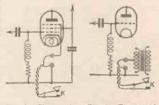
Fig. 3.—Placing the key in the cathode circuit. Fig. 4.—The method used for indirectly cheated valves.
