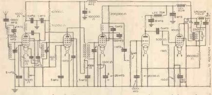
Fig. 1.—This 5-valve "straight" circuit has many interesting features which provide ample scope for individual experiment.
