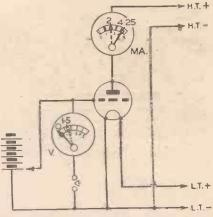
Fig. 1.—A simple circuit for testing battery triodes.
