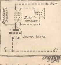
Fig. 2 .- An alternative connection to that shown in Fig. 1.
