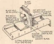
hows how this adjustment is made. The end of the base plate is left slightly longer, so that by placing this part of the tool on the edge of the work a regular and straight cut is made.
