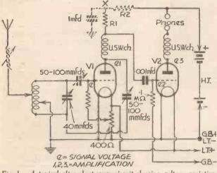
Fig. 1.- A lypical ultra-short-wave circuit showing voltage variation arises concerns the voltfrom stage to stage.
