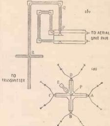
Figs. 1 and 2 .- Arrangement of aerial and feeder connections.
