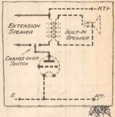
Fig. 3.—A change-over switch may be wired as shewn here, to change from built-in to extension speaker.
