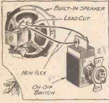
Fig. 5.-How to silence a built-in speaker.
