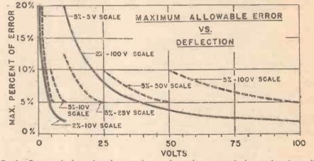
Fig. 3.—By using closely overlapped ranges, the error due to the necessity of taking readings for small deflections is eliminated. Note that the 5 per cent. meter represented by the dotted lines, in some cases has a lower allowable error than the 2 per cent. meter (solid lines).
