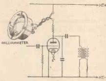
How to connect a meter in the anode circuit of a value.
