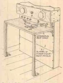
Fig. 2.—Table and test instruments supported in a convenient position.
