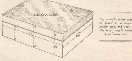
be housed in a simple wooden case, and a suitable design may be made up as shown here.
