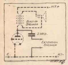
Fig. 1.-Standard output arrangement for a single extension speaker.
