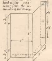
Fig. 7.—This is part of the B.F.O. screen. It is attached to the righthand screen in Fig. 4 and at the rear to Fig. 8.
