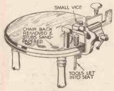
Fig. 1.-A disused chair converted for use as a small bench.
