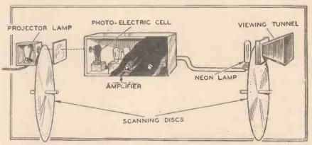
Fig. 2.—Simple television transmission and reception using disc scanners.
