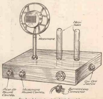
Fig. 2.—A front view of the finished amplifier.
