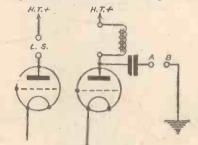
Fig. 2.—The ordinary types of loudspeaker connection.
