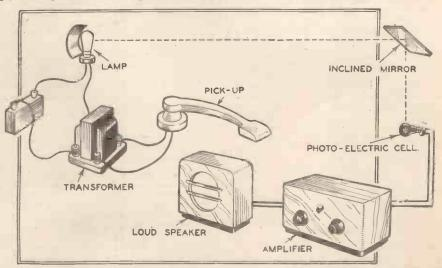
Fig. 1.—Using a beam of light for the transference of sound.
