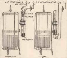
A simple mercury-operated time switch.
