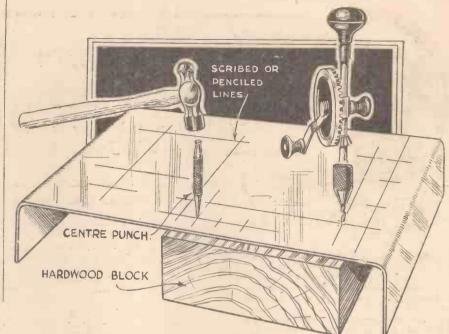
Fig. 3.—This illustration shows the steps in drilling a metal chassis. The positions are first marked with a scriber or pencil; next the centres are punched;
