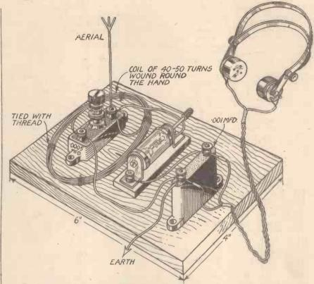
Fig. 1.— A simple crystal set which is suitable for reception of the local stations. It can be made in half an hour or less.
