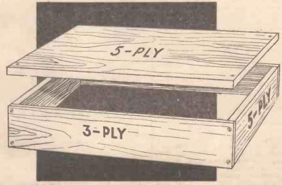
Fig. 5.—This shows a method of making a rigid and useful type of wooden chassis. .
