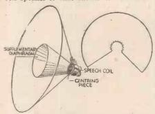
A simple dodge for improving high-note response in a moving-coil speaker.
