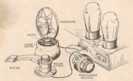
Fig. 1.—This shows the connections for a microphone and pick-up used together, and in conjunction with a potentiometer by means of which either can be faded in or out.
