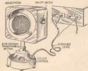
Fig. 3.—When using a microphone of the type which is supplied complete with transformer and battery the leads may be of almost any length, but must be screened.
