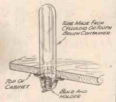
Fig. 1.—Method of fitting the bulb holders and covers to represent "neon" tubes.
