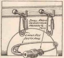
A novel use for safety-pins for keeping nuts-washers, etc., always at hand.
