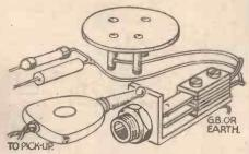
Fig. 2.—An alternative method of connecting the pick-up in circuit is to use a plug and jack.
