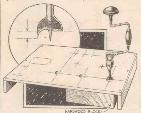
Fig. 1.—Showing the method of boring valve-holder holes with a centre bit. The bit must be sharp, and the tracing edge should project beyond the line of the cutter, as shown in inset.
