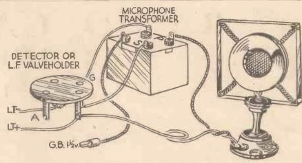
Fig. 2.—In some cases it is possible to energise the microphone by means of the L.T. battery if the connections are made, as shown, to the filament terminals of one of the valve-holders. In this, case the receiver switch also acts on the microphone.
