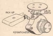
Fig. 3.—Simple volume control is carried out by means of a potentiometer.
