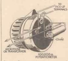
Fig. 4.—Connections for a volume control, which is required only when the microphone is not fitted with one.
