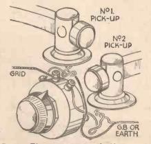
Fig. 4.-- This arrangement is preferable when two pick-ups are to be used.
