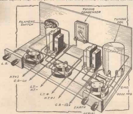
Fig. 2.—Here is a pictorial plan of the simplest type of Det. 2 L.F. receiver, which can be made from any odd components. Almost any coil may be used—even that shown in Fig. ), when medium-wave reception only is required.
