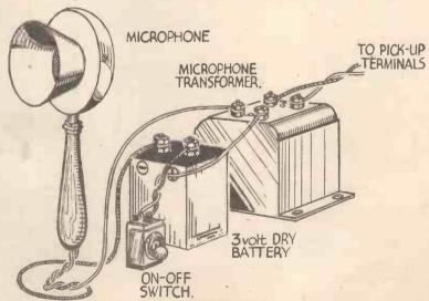
Fig. 1.—Showing how the simplest type of microphone is connected to the receiver or amplifier through a step-up transformer. Note the microphone switch. Note the connections of the dry battery and
