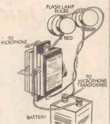
Fig. 2.—A simple method of connecting a microphone warning light is as shown here, where a two-pole change-over switch is used in the microphone-battery circuit.
