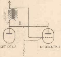
Fig. 1. — A coupling component may be eliminated in this manner.
