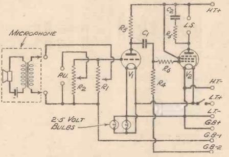
Fig. 3.—Circuit-diagram for the dual-purpose amplifier.
