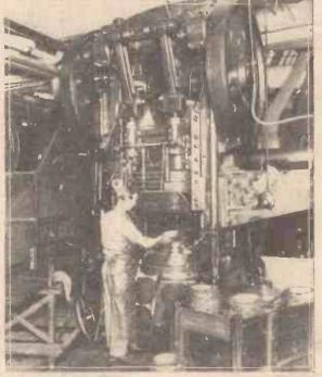
Stamping out the "Pan," or metal chassis, for H.M.V. loud-speakers on a 200-ton press.
