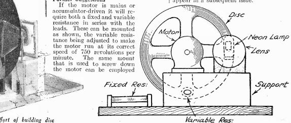
Fig. 2.—A rough layout of the disc model television apparatus.
