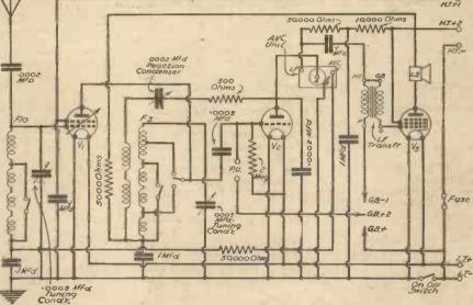
Theoretical circuit of F. J. Camm's amazingly successful receiver, with automatic fading compensation: "The Orbit."
