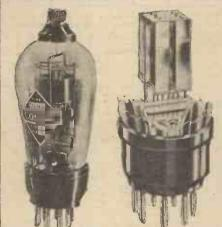
The Cossor DD/PEN. a double-diode variable-mu L.F. pentode evolved for true A.V.C.
