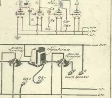
Fig. 1.—Tuned anode, detector, 2 L.F. stages without decoupling. Arrows indicating path of feed-back to grid of detector valve.
