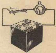
Fig. 3.—A milliammeter with a line resistance in series will act as a voltmeter.
