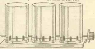
Fig. 8.—To avoid interaction the tuning coils are enclosed in cans. This is a 3-gang coil unit.
