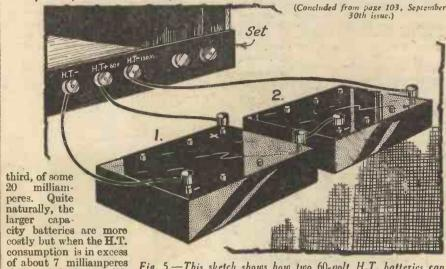
Fig. 5.—This sketch shows how two 60-volt H.T. batteries can be wired in series to effect an economy.
