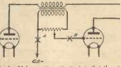
A very important type of test Fig. 6.- Make sure in continuity tests that there is not an alternative current path.
