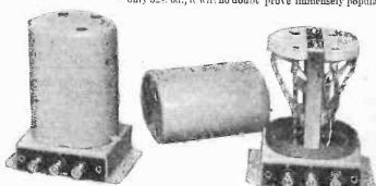
The new British Radiophone phone intermediate frequency transformer with screen removed to show construction.
