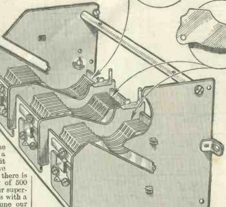
This illustration shows a three-gang condenser, with the top inset showing the special oscillator shaped plates.
