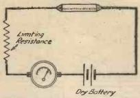
Fig. 5.- A milliammeter in series with a limiting resistance and small dry battery can be used to measure resistances.
