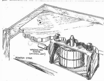
Marking out the hole in a radiogram cabinet for the winding handle.
