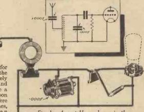
Fig. 1.—A variable condenser in the aerial lead.
