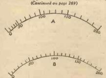
Fig. 4.—Comparison between scale of moving-iron and moving-coil instruments. A. Moving iron (crowded at bottom). B. Moving coil (equally divided).
