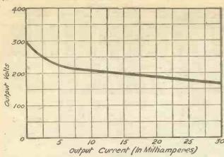
Fig. 4.—The above graph shows how the voltage output from an eliminator varies with the current drawn from it.
