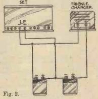
tor on charge is absolutely separated from the set, but it is a matter of a moment to change over plugs when required. is no risk of hum as in the arrangement with the D.P. double-throw switch which necessitated one lead from trickle charger going straight to L.T. terminal on the set. Having eight contact points in the case of the two plugs and sockets, against six in the case of the switch, enables one to com-pletely separate the circuits besides being instantly detachable.
