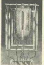
Fig. 1.—Electrode system of Cossor 41 MH, cut away to show heater.
