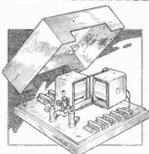
A Universal Distant-Con-trol Relay, manufactured by Messis, Bulgin. This costs 25s. and may be used with any type of receiver, D.C., A.C. or battery-operated.
