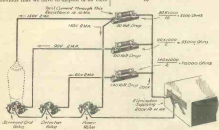
Fig. 5.—This illustrates the method of obtaining alternative anode voltages from an eliminator.
