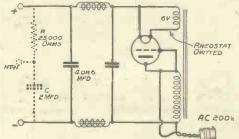
Fig. 2-Circuit diagram of a cheap H.T. climinator.
