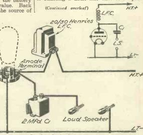
Fig. 2.—Choke filter output circuit.
