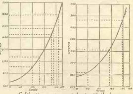
Calibration curves carried out with the buzzer wavemeter.
