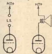
1. - AFig. 2.-Incorrect method simple output of coupling output valve to circuit. moving-coil speaker.
