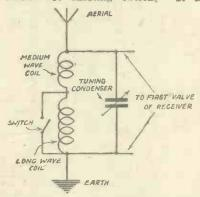
Fig. 6.—The circuit of a complete aerial tuner.
