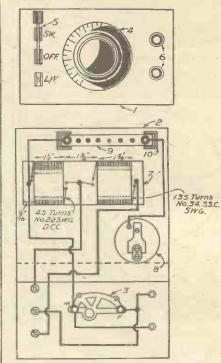
Panel and layout of a buzzer wavemeter.
