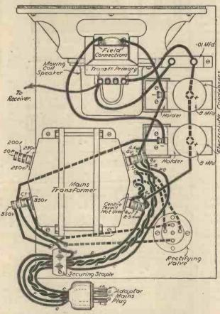
Fig. 2-Wiring diagram of the Mains Unit.
