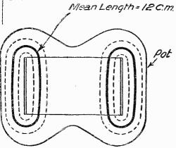
Fig. 2.—This diagram shows the arrangement of the magnetic field round a "potted" coil.
