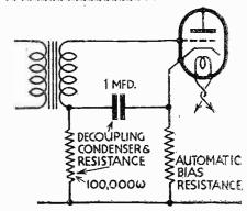
Fig. 3.—Complete decoupling has been added Before concluding, let us discuss the in this modification of the Fig. 2 arrangement
