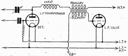
Fig. 22.—Method of feeding the L.F. valve through a transformer.
