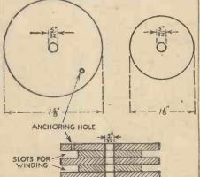
Fig. 2.—Showing wooden discs and method of assembly.
