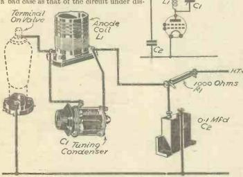
Fig. 4.—Decoupling the tuned-anode circuit.
