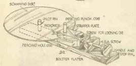
Device for punching holes in a scanning disc.
