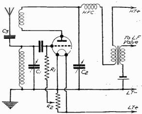
Fig. 2.—A modification of Fig. 1.—This is the throttle reaction control.
