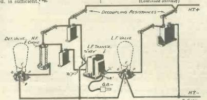
Fig. 13.—The addition of "decouplers" to stabilize a receiver.
