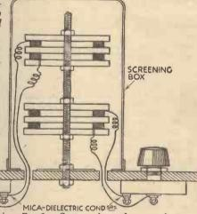
Fig. 3.—Section of complete transformer.
