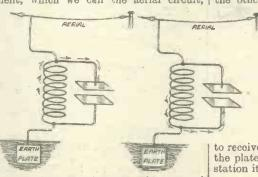
3,-Diagram illustrating the action of the transmitting and receiving circuits.
