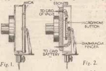
A pick-up made from a gramo. sound-box. Constructors will probably want to vary the range of their coils, but the details of the ones I have made may prove useful. The first coil consisted of four turns of
