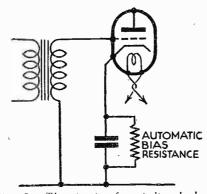
Fig. 2.—The circuit of an indirectly-heated power valve with automatic grid bias.
