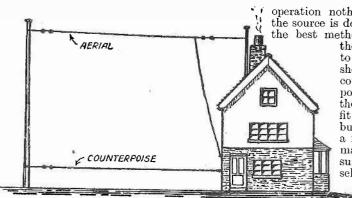
Fig. 5.—A counterpoise is sometimes useful in reducing interference.
