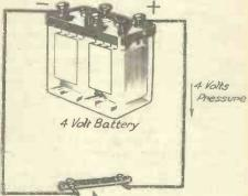
20hms Resistance Fig. 1.—This sketch illustrates the principle of Ohm's law.
