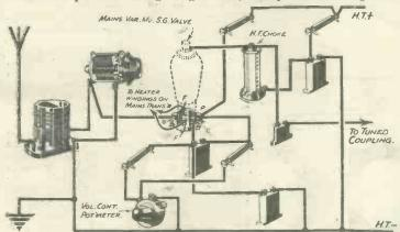
Fig. 12.—Using a variable-mu valve so that the biasing resistances carry the valve's own anode current.
