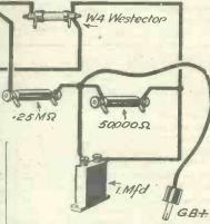
Fig. 1.—This sketch shows how the new components are connected to the output valveholder.
