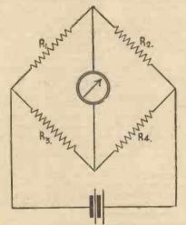
Fig. 1.—The circuit arrangement of a standard bridge.
