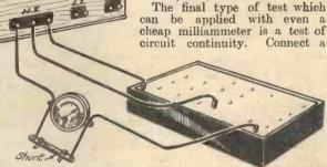
Fig. 4.—A shunt connected in parallel with a milliammeter measures its range.
