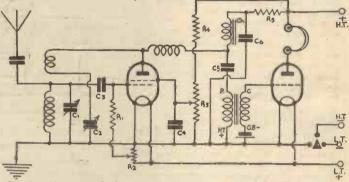
Fig. 1.—A very good short-wave circuit using choke fed L.F. coupling.
