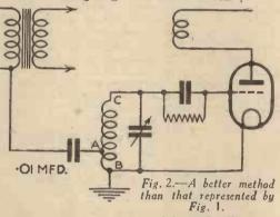
nection to the "top-end" of the grid-coil as shown. Fortunately, we have a way out of our difficulties. By arranging for a tap on our grid-coil we immediately reduce aerial damping. The arrangement (shown in Fig. 2), may be considered
