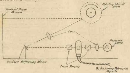
Fig. 2 .- The schematic arrangement and light beam path of the Visor-Teledrum.
