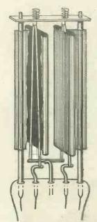
Fig. 4.—The internal con struction of the 442BU rectifier showing the tape filament.
