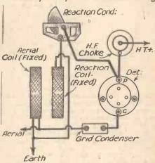
Fig. 10.—Connections for Reinartzor capacity L controlled reaction.
