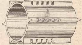
Fig. 3.-How a ribbed ebonite former may be slotted to accommodate the long-wave winding.
