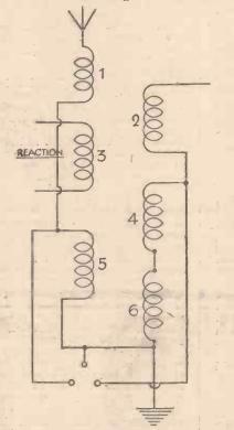
Fig. 6.—A selective dual-range arrangement. and correct operation in an old set. First is the matter of using correct voltages. Look up the maker's particulars, and see that you are working them all at correct voltages. If your output valve, say, is rated 100 to 150 volts, then see that it gets at least an honest 120, and then bias in proportion. Your detector voltage should be varied experimentally. Best results may lie between 40 and 70 volts. There is no point in overdoing
