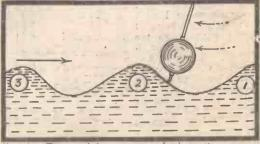
Fig. 6 .- The pendulum swinging back in time to meet the second wave.
