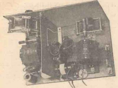
Fig. 4.—An early receiver employing a special type of low-loss coil.
