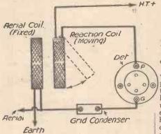
Fig. 9.-Connections for a swinging coil reaction circuit.
