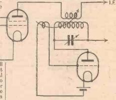
Fig. 6.—Using an S.G. valve as anode-bend detector.
