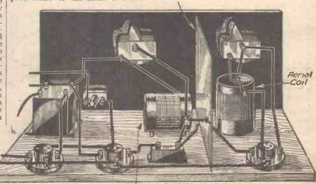
Tuned Anode Coil Fig. 11.—The kind of screening first used between large tuning coils of the solenoid type.
