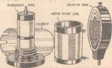
Fig. 9.—Different types of coils that may be used for "tuning" your set.
