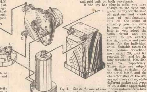
nections and components needed It will, of course, be un-for capacity-controlled reaction. derstood that the "aerial"
