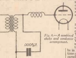
mains sets motor-boating does not always manifest itself; the trouble is present right from the start as a bad hum which no extra amount of smoothing will cure. In each of these cases adequate decoupling of the anode circuit will effect a cure.
