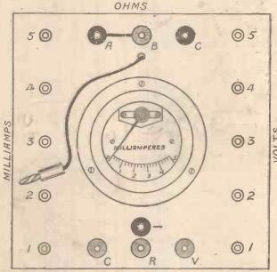
however, and that is—in case of doubt plug into socket No. 5 and gety some idea of the amount of current flowing, before coming down to the correct socket.
