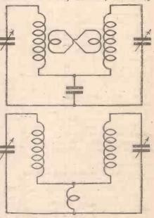
Fig. 4.—Inductive coupling between circuits.
