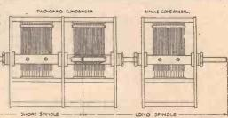
spindle is gripped by one of the grub screws of the middle condenser. The resultant assembly is quite rigid, and has remained so for some time.—F. J. HAYWARD (New Malden).
