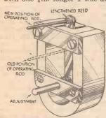
reed below, instead of above, the bobbin and pole pieces. This gave me twice the distance from the pivot and correspondingly greater movement of cone, resulting in a vast improvement
