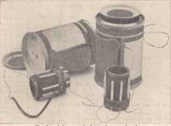
Fig. 1.—A home-made form of screened coil.
