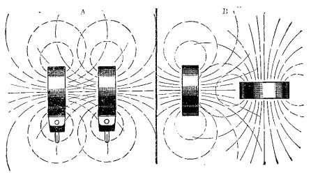
Fig. 1.-Showing the shape of the electro-magnetic field of coils of the usual plug-in type.
