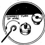
Bend the wire in a clockwise direction, as shown, and the terminal nut will then grip the wire tighter round the thread. How to Commence
