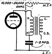
Fig. 5.—How to fit a decoupling resistance and condenser to stop motorboating.
