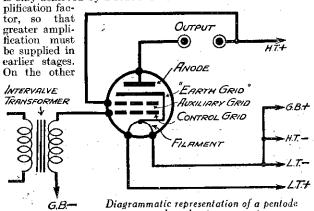
output valve, showing connections.
