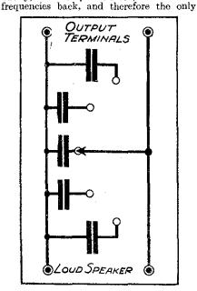
Fig. 1.—How to arrange a number of fixed condensers across the output terminals to vary the tone.
