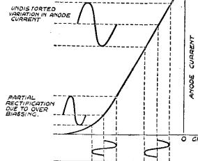
Showing relation between the grid voltage and the anode current in a valve and indicating correct biassing and how distortion is introduced by over-biassing.
