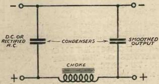
Fig. 2.—A choke connected up in a typical smoothing circuit.
