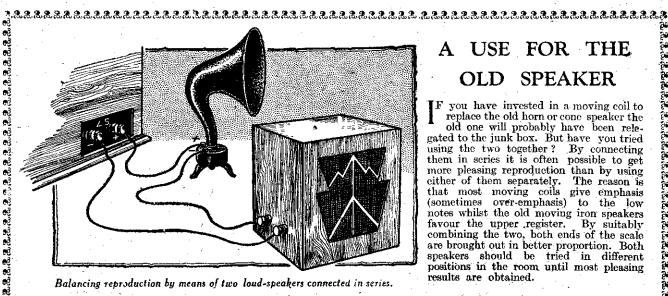
Balancing reproduction by means of two loud-speakers connected in series.
