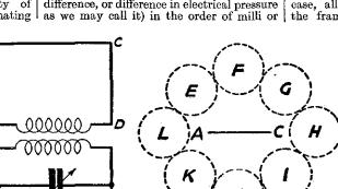
Fig. 3.—The frame aerial with its small coil coupled to the main tuning circuit.
