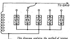
This diagram explains the method of joining up the condensers. The diagram also shows how a number of semi-fixed condensers may be connected up to enable the scheme described in this article to be carried out.
