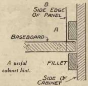
although most baseboards are of plywood these do not always remain true—it may be of interest to readers to know that quite a lot of makes of plywood "wind." (This term "wind" is used to denote a diagonal twist). It is a far better scheme to brad and glue another fillet (A) above (or below) the first one at such a distance that the baseboard will slide into cabinet between the two strips, thus holding the baseboard true and firmly, but also allowing of easy removal. One should note that
