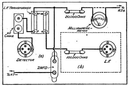
Fig. 3.—A decoupling resistance in the anode lead, and a resistance in the grid lead to cure instability.
