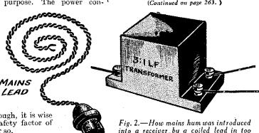
into a receiver by a coiled lead in too close proximity to a transformer.
