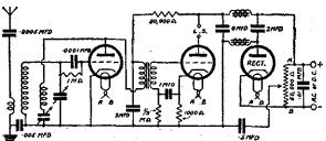
Fig. 4.—Circuit diagram of the Ostar Universal two-valve receiver,
