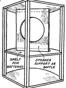
Fig. 2.—The main framework of the corner
