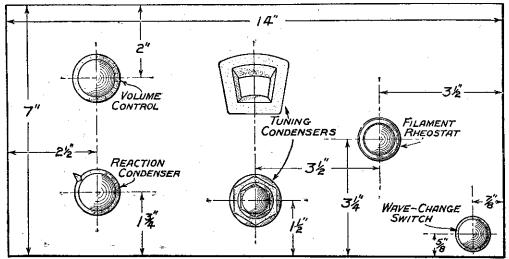
Template for marking position of holes on the Camco Ambassador Cabinet front.
