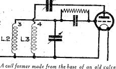
REACTION COIL and (right) a circuit diagram using the four-pin coil.
