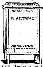
Fig. 8.—A radio-gram cabinet containing aerial and earth blates.
