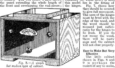
If, however, If, however, you prefer the ends to overlap the front and back, there is no reason why should not. In this case the rails fitted to the front n d back as stops to prevent the ends
