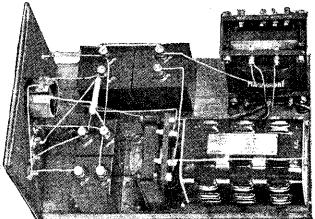
A plan view of the A.C. eliminator, showing the layout of the components and the wiring.
