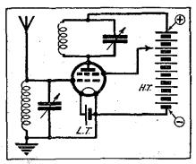
■ Fig. 3.—A screen-grid valve employing tuned-anode coupling.
