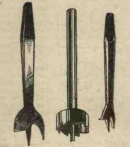
Fig. 5.- Centre-bits, and a panel cutter,
