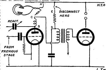
Fig 9.—How to test for "crackling" noises. To test the H.F. and detector stages disconnect H.T. from E and join phones across A and B. To test H.F. choke as well join phones across A and C. To include transformer join them across A and D. To include decoupling resistance join across A and E.
