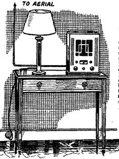
Fig. 8—One cause of hum is the actial, earth or speaker leads, running parallel to the supply mains.
