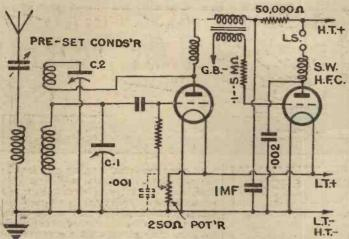
Fig. 2.- A good two-valve short-wave circuit.
