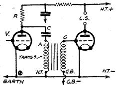
Fig. 2.—The method of parallel-feeding a transformer.
