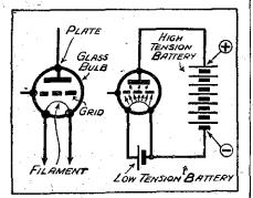
Fig. 1—The wireless valve, and a diagram of the way in which the electron stream is emitted.
