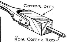
How to fit a small bit to your soldering iron.
