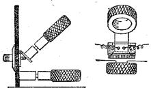
Converting plug-in coils to panel mounting with a fine adjustment.
