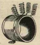
Fig. 1.—The single layer wound solenoid coil.
