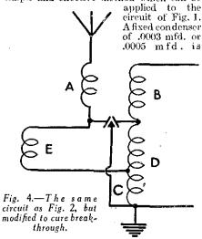
placed across C. This again increases the wavelength of the aerial coil without increasing the coupling. In this way the selectivity on the long waves still remains
