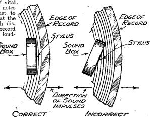
musical scale are not recorded at the same The "tracking" angle—which was fully explained in a recent strength as the higher notes issue. Note how the sound-box or pick-up must be parallel with the sound grooves.
