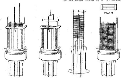
Steps in the construction of a modern screen-grid Cossor valve.
