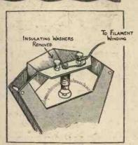
A neat method of fixing a bulb for an illuminated dial.
