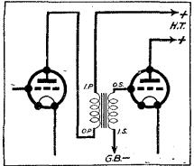
Fig. 2a.—Transformer primary directly in anode circuit.
