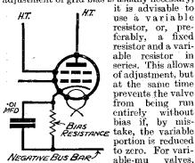
able-mu Fig. 5.—The biasing re-where continusistance arranged in the ously adjustable cathode lead of an S.G. bias is required, the resistance
