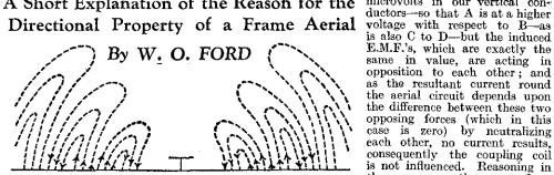
Fig. 1.—How the lines of stress radiate.
