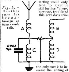
the series aerial condenser and make up for the reduced selectivity by decreasing the coupling between the primary and second-ary circuits. If the coil is a home-made one, this can easily be arranged, either by reducing the number of turns in the tapped portion C, in the case of Fig. 4, or by plac-ing the windings C and D farther apart, in the case of Fig. 5.
