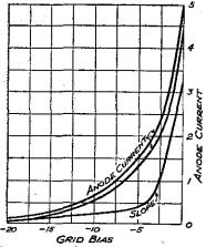
The characteristic curve of the variable mu valve. Note the long, gentle slope caused by the irregularly spaced grid.
