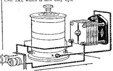
Method of controlling the volume from the input side of a wireless circuit.
