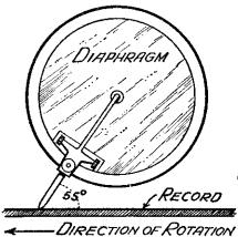
The correct angle for a needle-with either ordinary acoustic sound-box or electric pick-up.
