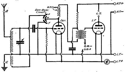
Fig. 2.—Circuit of a two-valve receiver.
