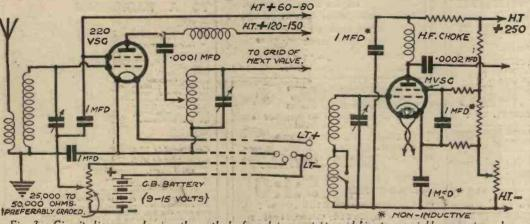
Fig. 3.—Circuit diagrams showing the method of applying variable grid bias to a variable mu mains valve and one of the battery type.
