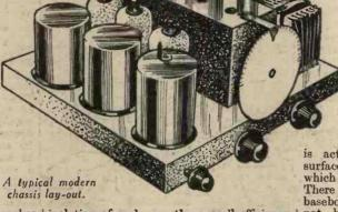
isolation of each one, the overall efficiency is much greater than that of the unscreened coils. Furthermore, as the earthed screen surrounding the coil completely isolates it from external influences, two or more coils may be tuned by two condensers joined together (or ganged), the circuits remaining matched over the complete tuning scale. This, then, is one of the important features of the chassis built set.
