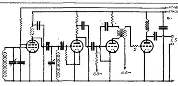
Fig. 7.-A typical four-valve circuit showing the method of inserting the decoupling resistances.
