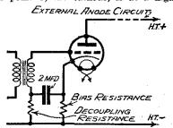
The arrangement of Fig 1 with a de-coupling circuit added.
