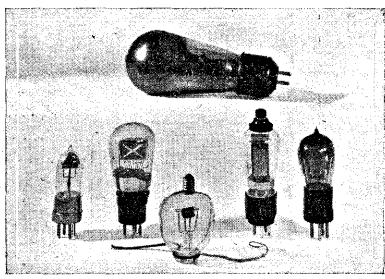
Fig. 2.—A group of Cossor valves indicating various stages in development. Top: Super-power valve of 60-Watt dissipation. Bottom row (left to right): (1) 1921—.6 power valve, Stentor class. (2)—Modern pentote. (3)—1916 valve of peculiar construction. (4)—Modern mains S.G. valve (5) 1923—.3 amp. kalenised filament.
