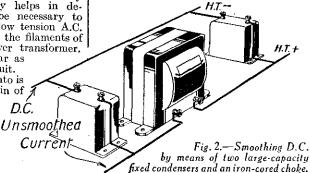
to the choke is a great deal more smooth. The choke in its turn does the work of opposing current fluctuations, passing on a still more steady flow to the second condenser; this is the final reservoir from which the high tension is derived for the set. Usually the inductance value of the choke is not less than 30 henries and the capacity of condensers at least four micro-farads each.
