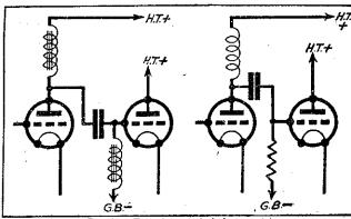
Fig. 3.—Two forms of choke coupling.
