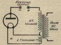
Fig. 1 .- The "diode," or two-electrode valve, used as a rectifier in an A.C. mains set.
