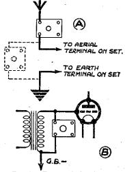
Fig. 2.-Two methods of using the control: (A) on the aerial circuit, and (B) across a transformer.
