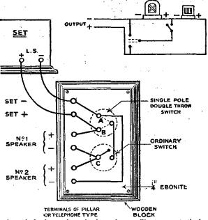
A method of switching loud-speakers. insulated wire at back of ebonite. Wir A, B and C. Glazite or similarly Wiring looped in at points
