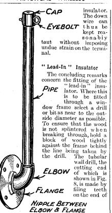
Fig. 8.—Showing metal fittings for making a short mast.
