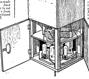
Fig. 6.—Rear view of the completed cabinet, showing set and batteries.
