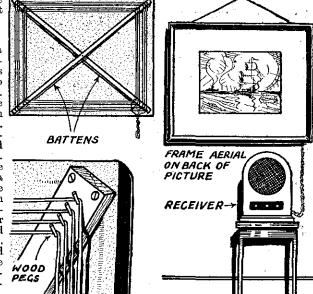
Figs. 5, 6 and 7.—A picture frame can be easily adapted to accommodate an aerial.
