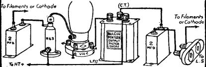
A new L.F. Choke specially designed for use with Pentode valves, electrically centre-tapped to enable a step-down ratio of 2-1 to be obtained. Fitted in new universal mounting case for either chassis (inverted) or baseboard mounting, it is beautifully finished in frosted aluminium with insulated terminals.
