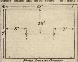
Fig. 2.- How to drill the panel.
