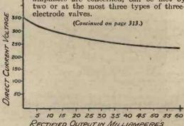
RECTIFIED OUTPUT IN MILLIAMPERES Fig. 3. — Typical performance curve of a rectifier valve.
