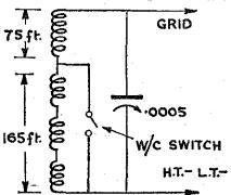
Fig. 1.—Diagram illustrating reply concerning frame gerial windings.
