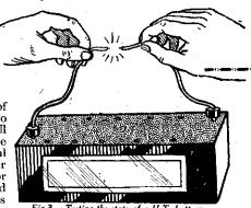
Fig 3.—Testing the state of a H.T. battery.
