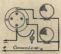
Two methods of using a valve holder as a switch.
