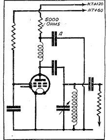
Fig. 4.-S.G. stage decoupled.
