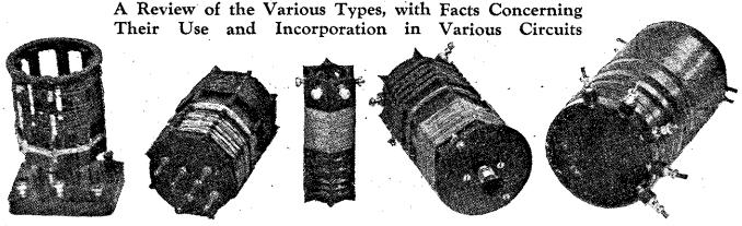
A set of home-made tuning coils: Reading from left to right the coils are: A short-wave tuner with 6-pin base; a broadcast tuner with 6-pin base; a smaller dual-wave tuner suitable for use in screen-grid receivers; a broadcast tuner with built-in wave-change switch, and another broadcast tuner for baseboard mounting. The first coil shown is wound on a skeleton former, the second, third, and fourth use ribbed ebonite formers, and the fifth is wound on a paxolin tube.
