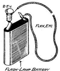
Fig. 1.—The simplest form of tester.
