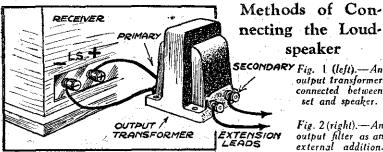
speaker SECONDARY Fig. 1 (left).—An output transformer connected between set and speaker.
