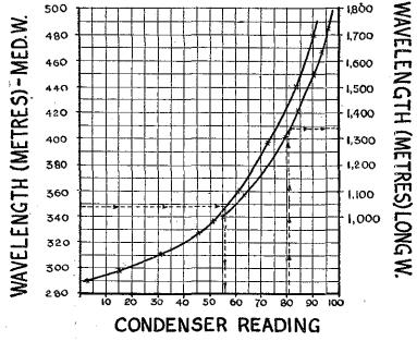
Fig. 5.- How to draw a calibration chart.
