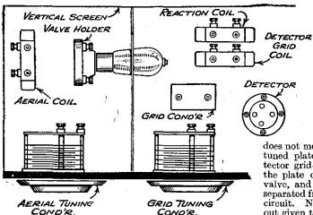
Fig. 1.—The layout of the H.F. stage.
