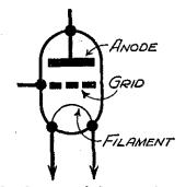
Fig. 3.—Conventional diagram of a three-electrode valve, indicating the essential parts.
