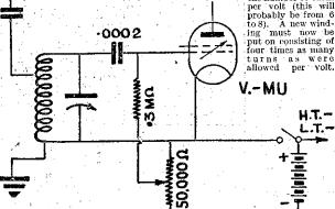
Fig. 3A.—The substitution of a variable mu value in a single circuit aerial tuner.
