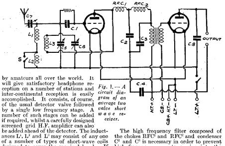
The high frequency filter composed of the chokes RFC<sup>1</sup> and RFC<sup>2</sup> and condenser C<sup>2</sup> and C<sup>3</sup> is necessary in order to prevent high frequency currents passing into the low frequency amplifier. This filter may take various forms but it is essential that the condensers remain of small value, otherwise the low frequency response characteristics of the receiver will be considerably altered.
