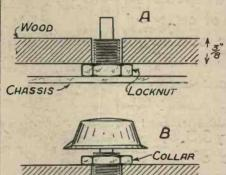
CHASSIS-Recessing a panel to take back nuts on components.
