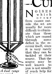
frame aerial that reason. The usual noises experienced are crack-ling and similar noises due to electrical machinery, mains hum, atmospherics, and heterodyne whistles.
