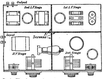
Fig. 4.—When the input and output ends of the receiver come close together the set should be screened as shown.
