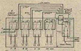
Showing general arrangement for an experimenter's switchboard.
