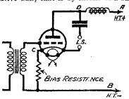
—A resistance inserted in the cathode lead of an indirectly-heated valve.
