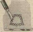
ary type of iron Fig. 11.—Trimming a hole in a panel with a pen-knife.
