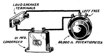
Fig. 10-A high-note filter—a care for whistle, caused by heterodyning.
