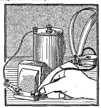
A simple method of testing with phones and a dry battery.
