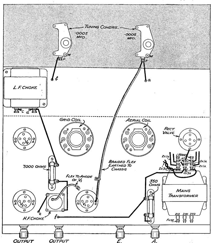
Above-Chassis Wiring Diagram of the Mains Express Three.
