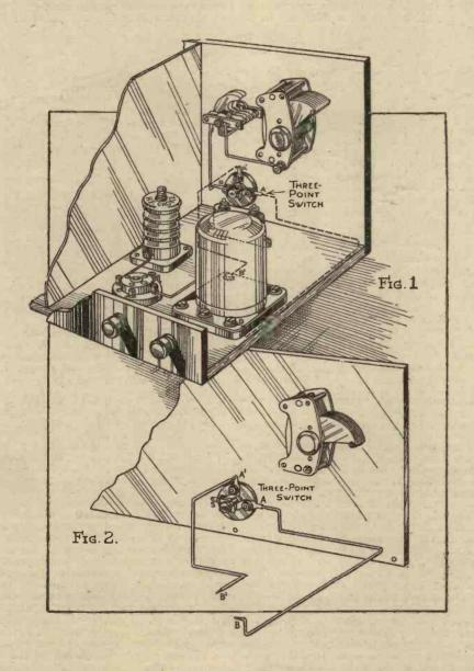
the remaining wiring is completed. Sometimes, however, these latter joints are very awkward to get at, especially with a hot soldering iron. Moreover, one slip may mean serious damage to a component, and I have myself often ruined a choke or coil trying to solder such joints. For instance, in the accompanying diagrams it would be difficult to solder a piece of wire to the switch S without doing damage to the adjacent components (Fig. 1). If the wires
