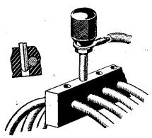
Simple method of tapping short-wave coils.
