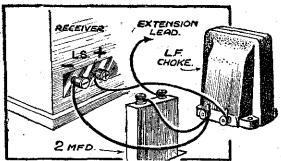
UITE a number of wireless listeners are under the impression that because the loud-speaker, when it is purchased, is fitted with connecting cords about six feet long it must be joined to the loud-speaker terminals of the set by those cords and placed as near to the set as possible. This is not the case by any means, and if you are doing this you may not be getting the best from your speaker.
