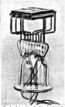
Fig. 1.—Internal construction of a typical battery-heated three-electrode valve.
