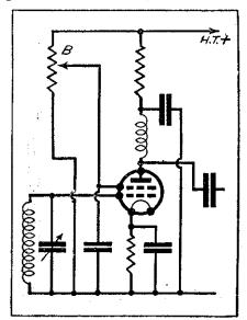
Fig. 5.—With the usual arrangement of a mains set the potentiometer acts as a decoupler.
