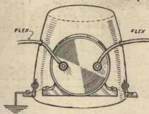
An efficient improvised screen for small H.F. chokes.
