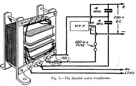
alternatively they may be bought readymade in the form of strong castings from the firms mentioned below. The drawing will need no explanation, whilst the method of fitting the clamps is clearly shown in Fig. 3. This latter drawing also shows the paxolin (or ebonite) terminal strips. These are fitted under the heads of the clamp bolts, and the leads from the spool are brought up to, and soldered to, the terminals.
