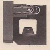
A paper clip used to repair one of the plastic tabs that secure Pace front panels.
